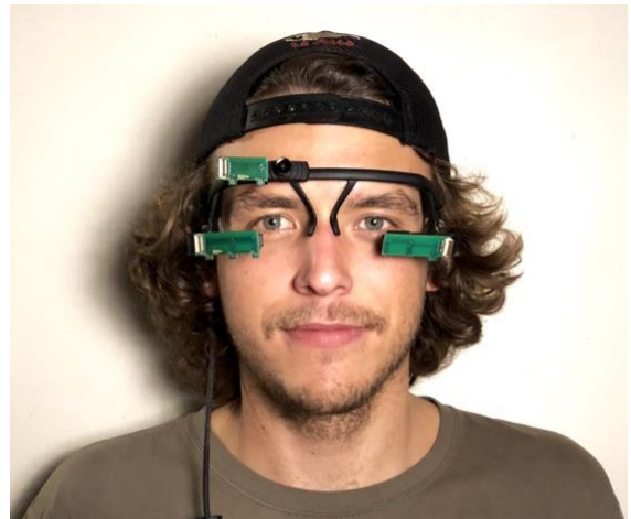
Figure 2. A Pupil Labs head-mounted VOG device [7] with custom PCBs added onto the backs of the standard eye-tracking cameras.
