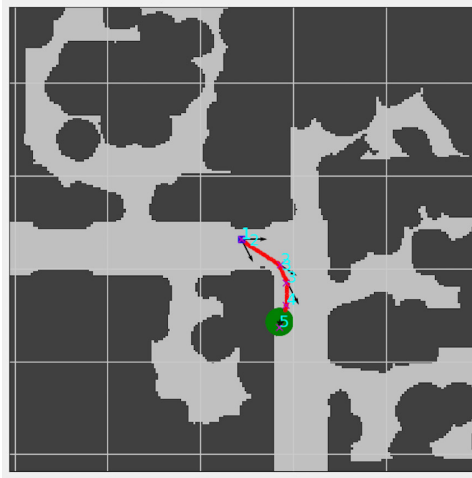
Figure 1: Top view of our method: The robot moves from start (blue dot) to goal (green circle), periodically producing new waypoints (cyan) that guide it towards the goal while avoiding collision with obstacles (dark gray).
