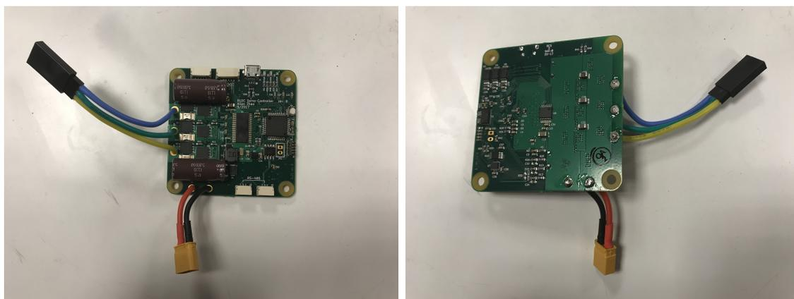
Figure 3.2: Assembled motor controller board (front and back)
