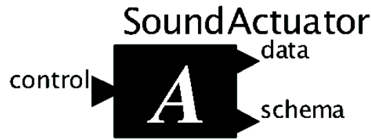
Figure 3.6: The actor interface for a ControllableSensor accessor like SoundActuator.
