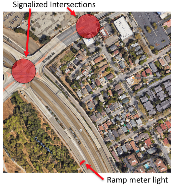
Figure 5.16: Freeway-arterial interaction at the intersection studied by Su et al. [85]. A long freeway ramp is actuated by a ramp meter that sets a rate that vehicles may enter the freeway. During periods of high congestion on the freeway, this rate decreases and the vehicle queue may spill back onto the signalized intersections upstream. Satellite Image Source: Google Maps.
