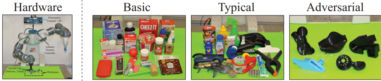
Figure 2.5: (Left) The experimental setup with an ABB YuMi equipped with a suction gripper. (Right) The 55 objects used to evaluate suction grasping performance. The objects are divided into three categories to characterize performance: Basic (e.g. prismatic objects), Typical, and Adversarial.
