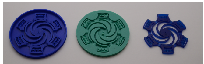
Figure 7: from left to right: 3-D printed negative of the mold; silicone mold itself; polyurethane part of the wheel.
