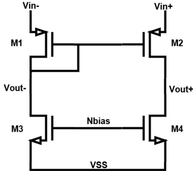
Figure 3.4: Schematic of the amplifier-based comparator controlling the gates of the PMOS of the rectifier.
