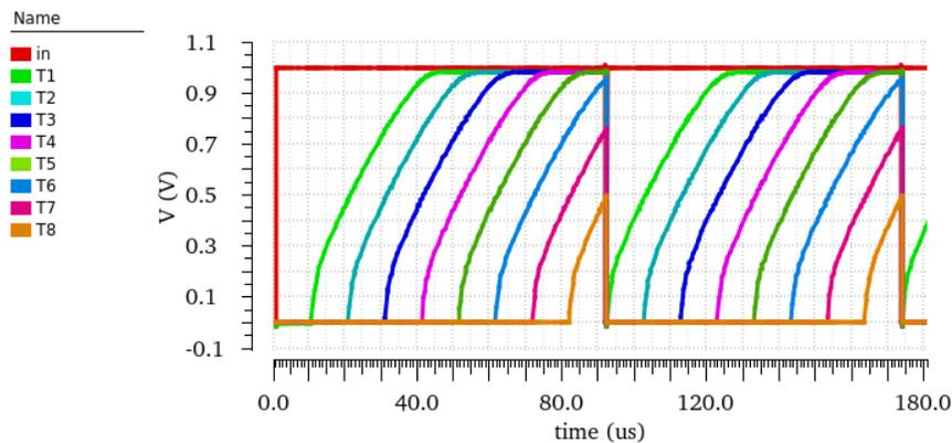
Figure 3.14: The TDC buffer chain rises until T8 is high. When T8 is high, the input becomes low to pull all the buffers' output to low. Once T8 is low again, the next cycle starts.
