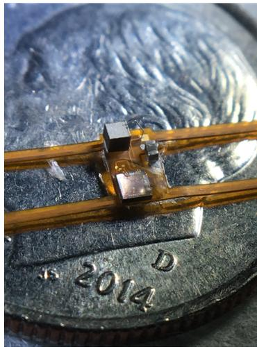
Figure 1.2: The photo of the StimDust mote on top of a dime. The three components on the mote from top to bottom are piezocrystal, 0201 capacitor, and the IC. [11]
