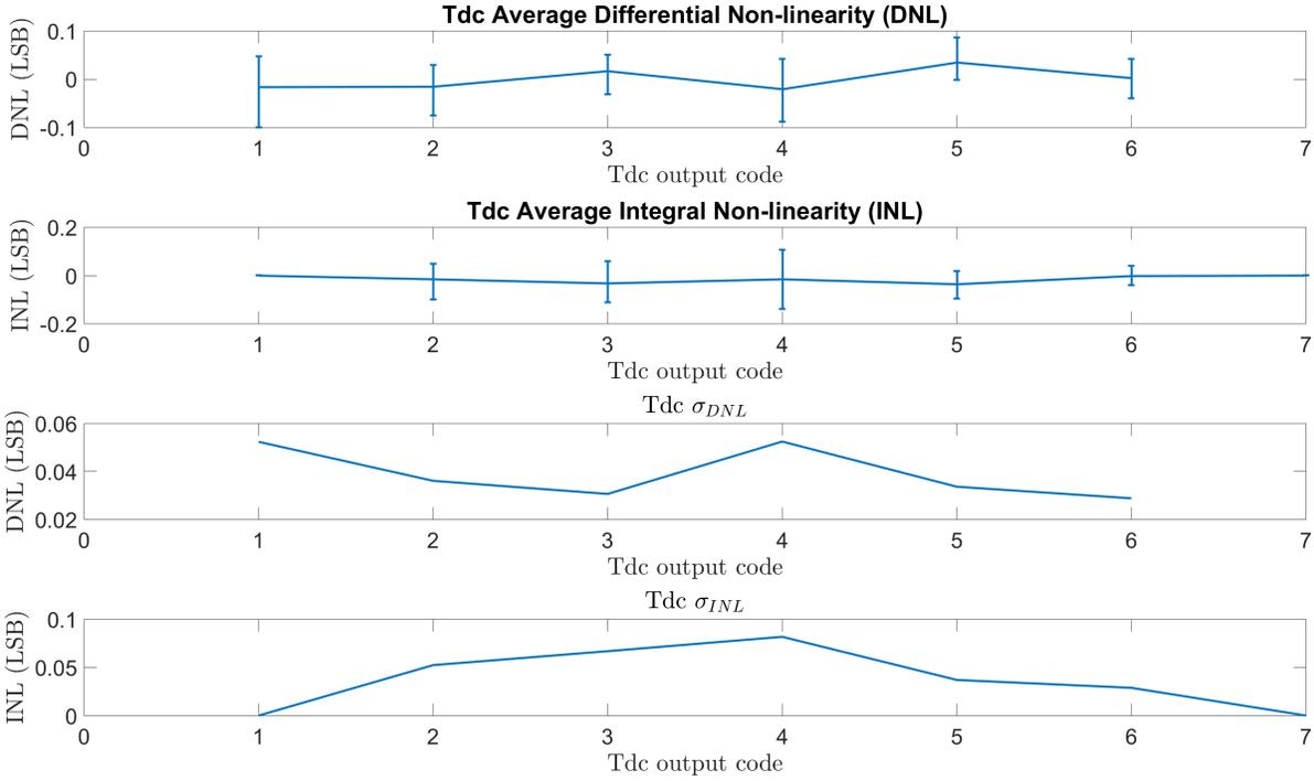
Figure 5.6: The nonlinearity of the Tdc. The error bar shows the range of DNL and INL across the five chips.
