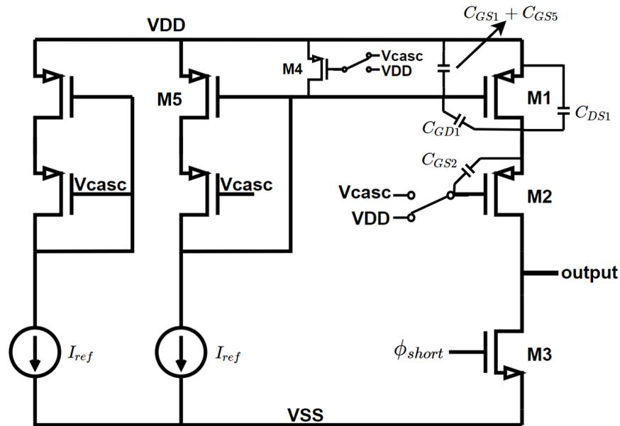
Figure 3.15: The schematic of the cascode current source being used in the DAC. The parasitic capacitors that is responsible for current peaking are also shown.
