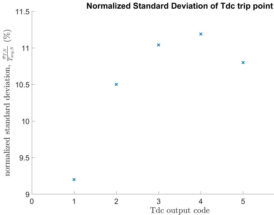
Figure 5.8: The standard deviation of the step size of TDC at each level, normalized by the average step size at that level.
