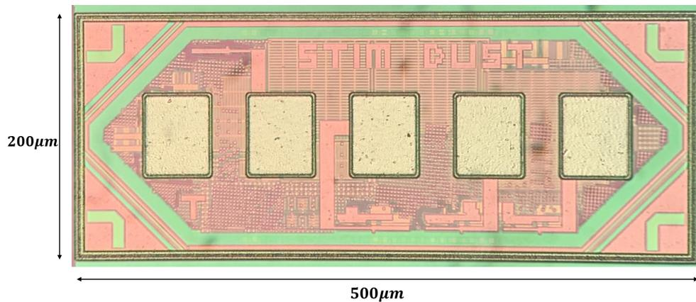
Figure 5.1: The die photo of the chip.
