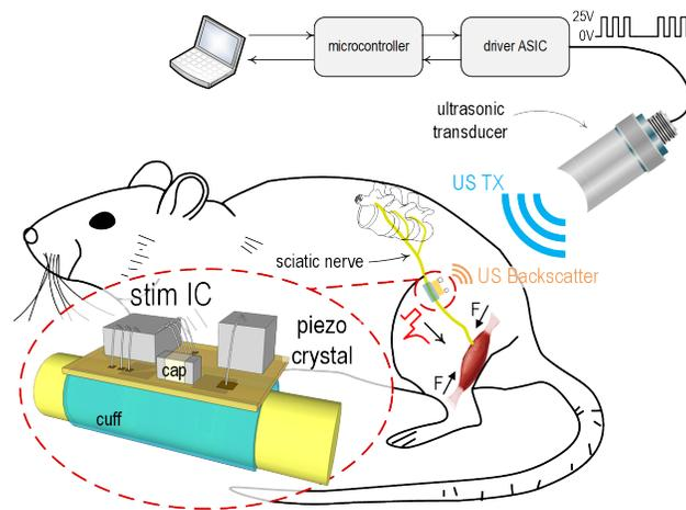
Figure 1.1: The system of the StimDust. The StimDust mote is cuffed to the sciatic nerve. External ultrasonic transducer is used to control and monitor the stimulation.
