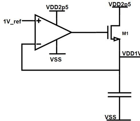
Figure 3.8: Schematic of the LDO
