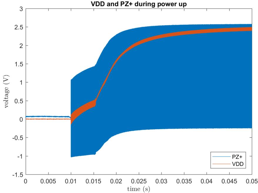
Figure 5.4: The waveform of the VDD of one chip during power-up measured by the oscilloscope.
