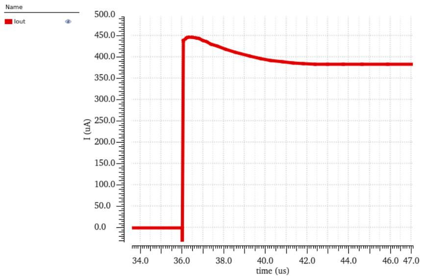
Figure 3.16: The simulation result showing the peaking of the output current. The initial overshoot is caused by the first spike. After that the second spike kicks in.
