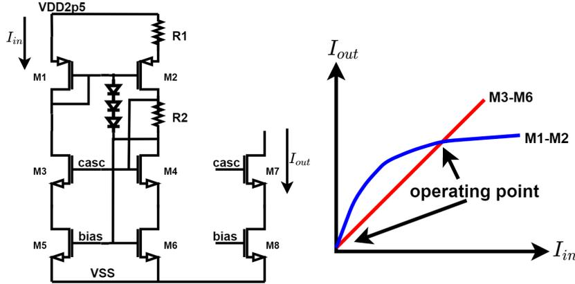
Figure 3.9: Schematic of the current reference circuits, and its input and output relation
