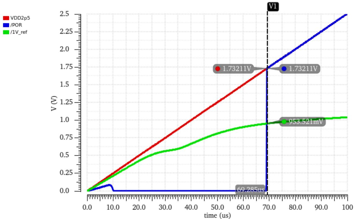
Figure 3.7: Simulation result of POR. The POR is high and  $1V_{ref}=953mV$  when  $VDD2p5=1.73V$
