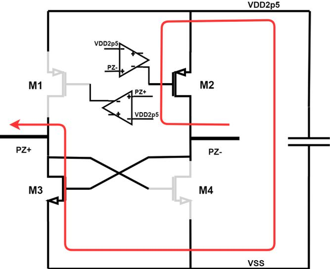
Figure 3.3: Signal path of the active rectifier when  $PZ- > PZ+$ . The transistors in gray are off. The transistors in black are on.
