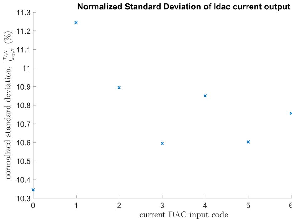
Figure 5.9: The standard deviation of the step size of the current DAC at each level, normalized by the average step size at that level.
