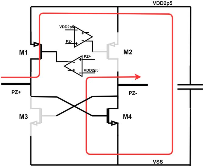
Figure 3.2: Signal path of the active rectifier when  $PZ+ > PZ-$ . The transistors in gray are off. The transistors in black are on.
