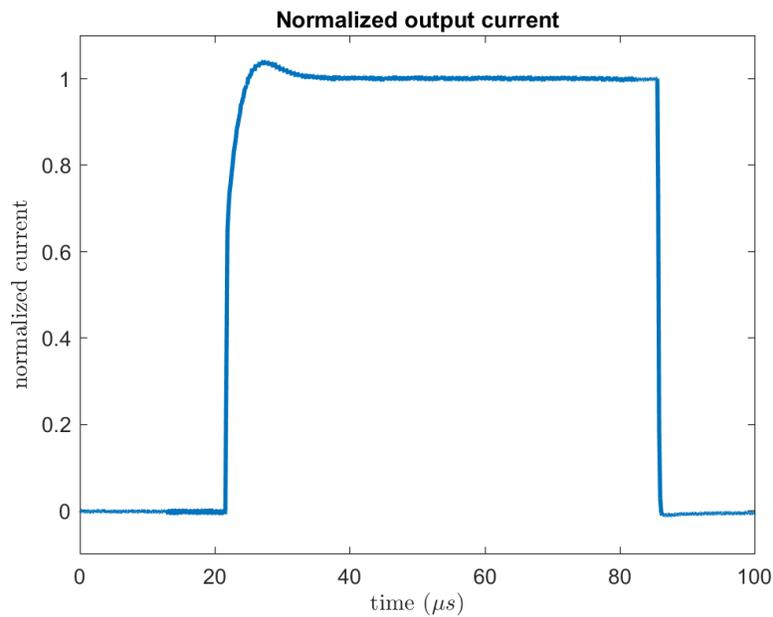
Figure 5.11: The waveform of the maximum current output normalized by the static current amplitude. The peaking is less than 5% in this example.
