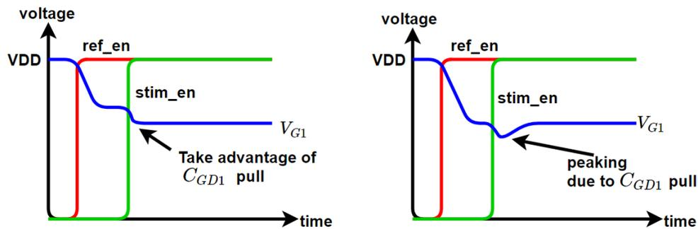
Figure 3.17: The M4 is used to bias  $V_{G1}$  slightly higher than its desired voltage to limit the peaking due to coupling from  $C_{GD1}$
