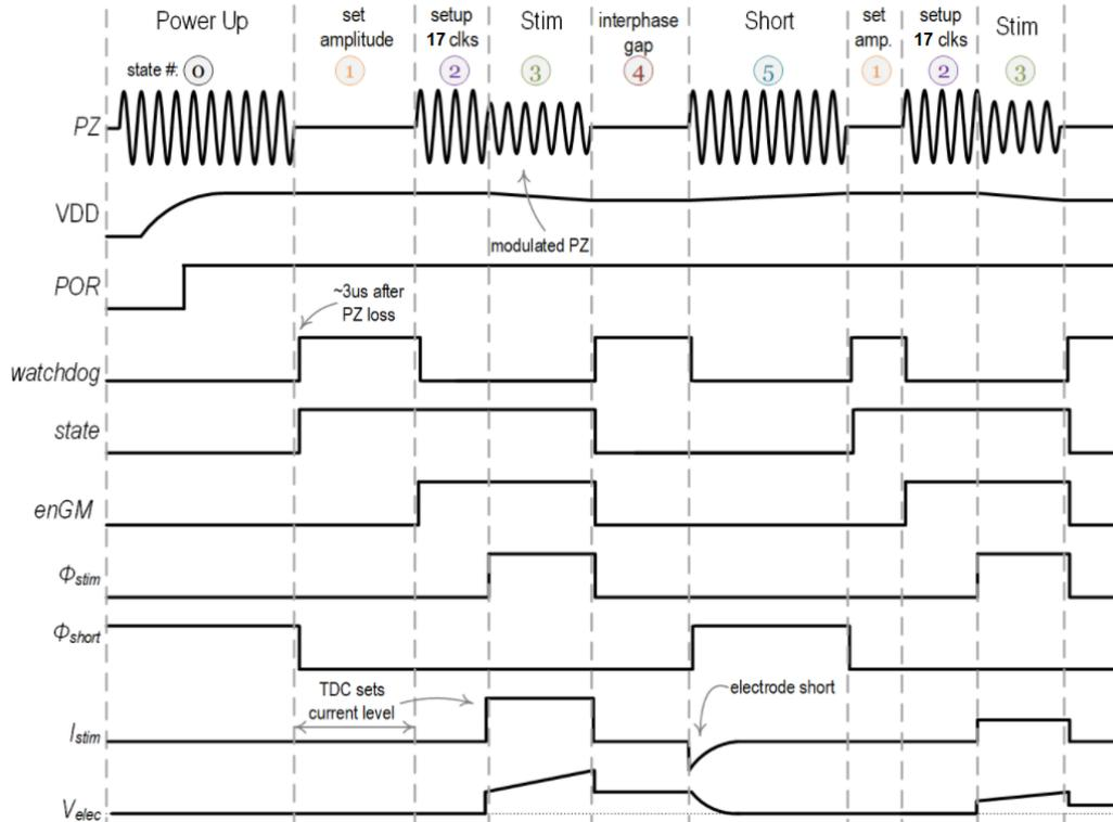
Figure 2.1: Timing diagram of the protocol
