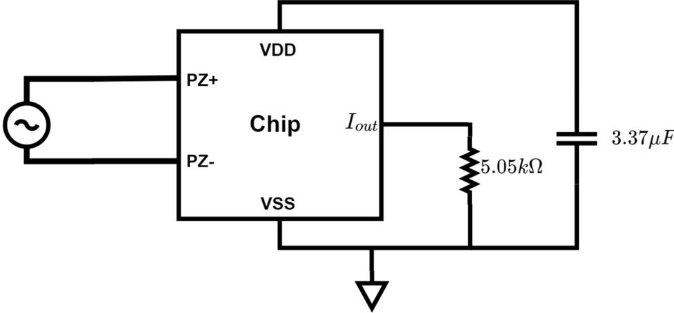
Figure 5.2: The test setup for functional testing.
