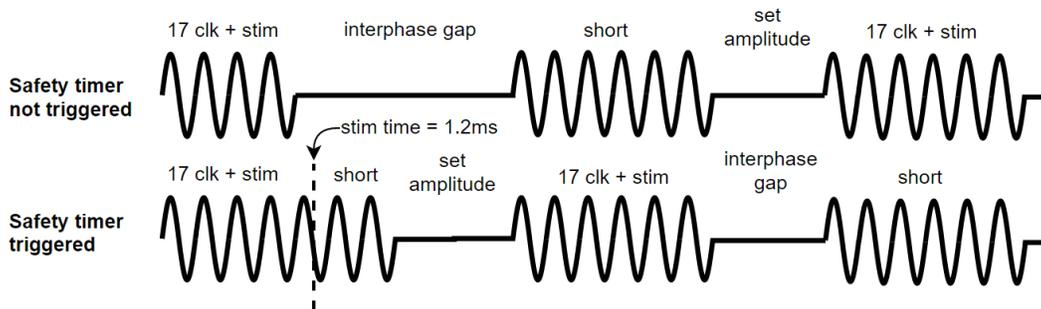
Figure 2.2: Timing diagram to demonstrate the states after triggering safety timer.
