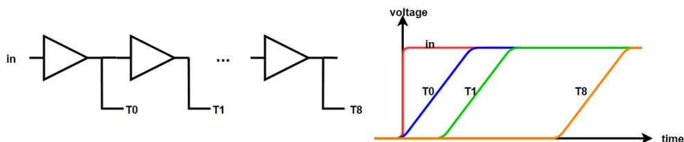
Figure 3.11: Timing diagram of the TDC when the input switches from low to high.
