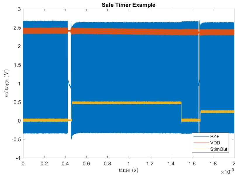
Figure 5.10: The waveforms example showing that the safety timer stops the stimulation after 1.04ms. The state of the chip is flipped such that the next pulses of ultrasound immediately starts the stimulation.
