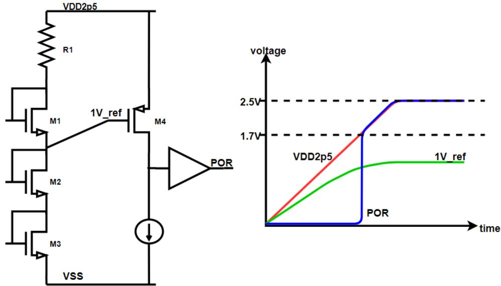
Figure 3.6: Circuit for  $1V_{ref}$  and  $POR$ , and their corresponding voltages as  $VDD2p5$  slews up
