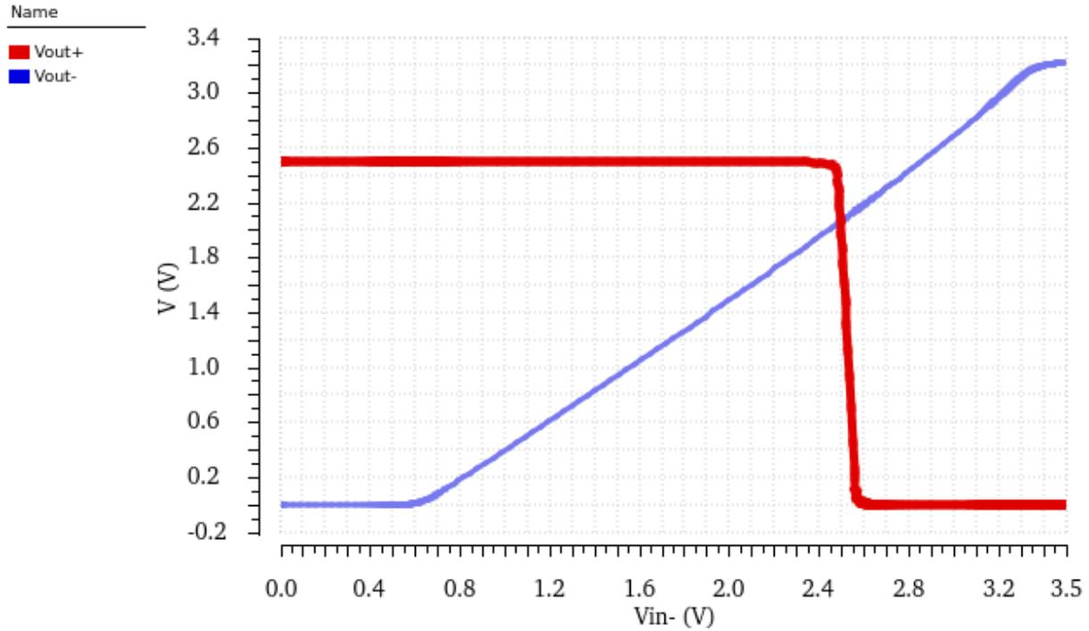
Figure 3.5:  $V_{out}^+$  and  $V_{out}^-$  vs  $V_{in}^-$  at  $V_{in}^+ = 2.5V$
