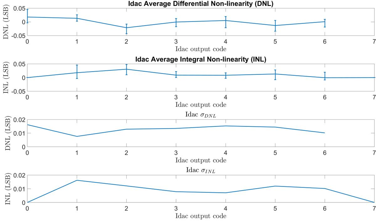
Figure 5.7: The nonlinearity of the Idac. The error bar shows the range of DNL and INL across the five chips.
