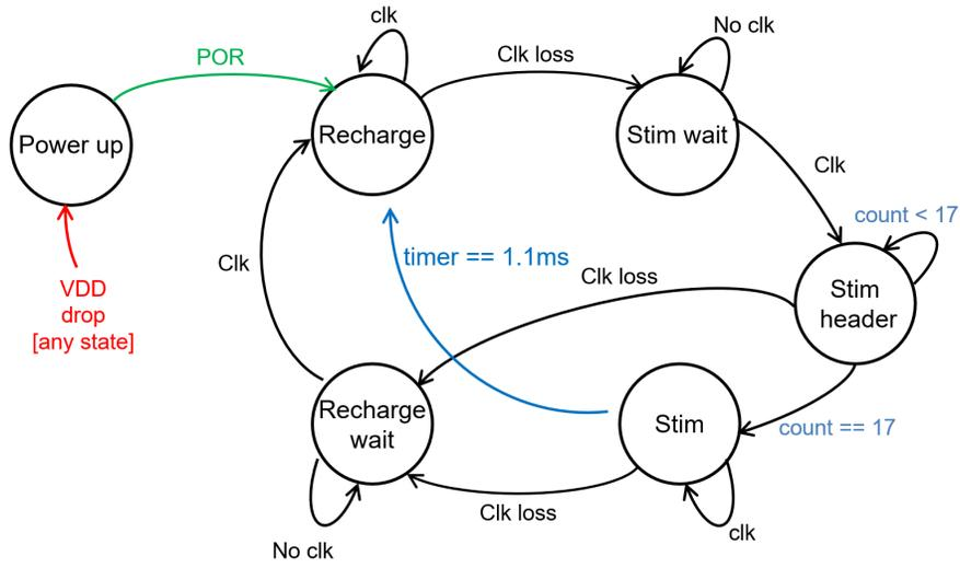
Figure 2.3: Finite state machine of this chip. The changes are highlighted in blue in the figure.
