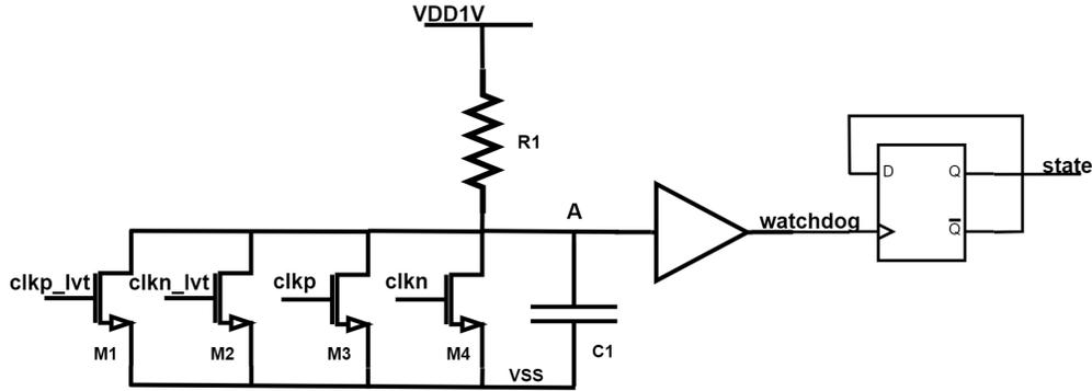
Figure 3.10: Schematic of the watchdog
