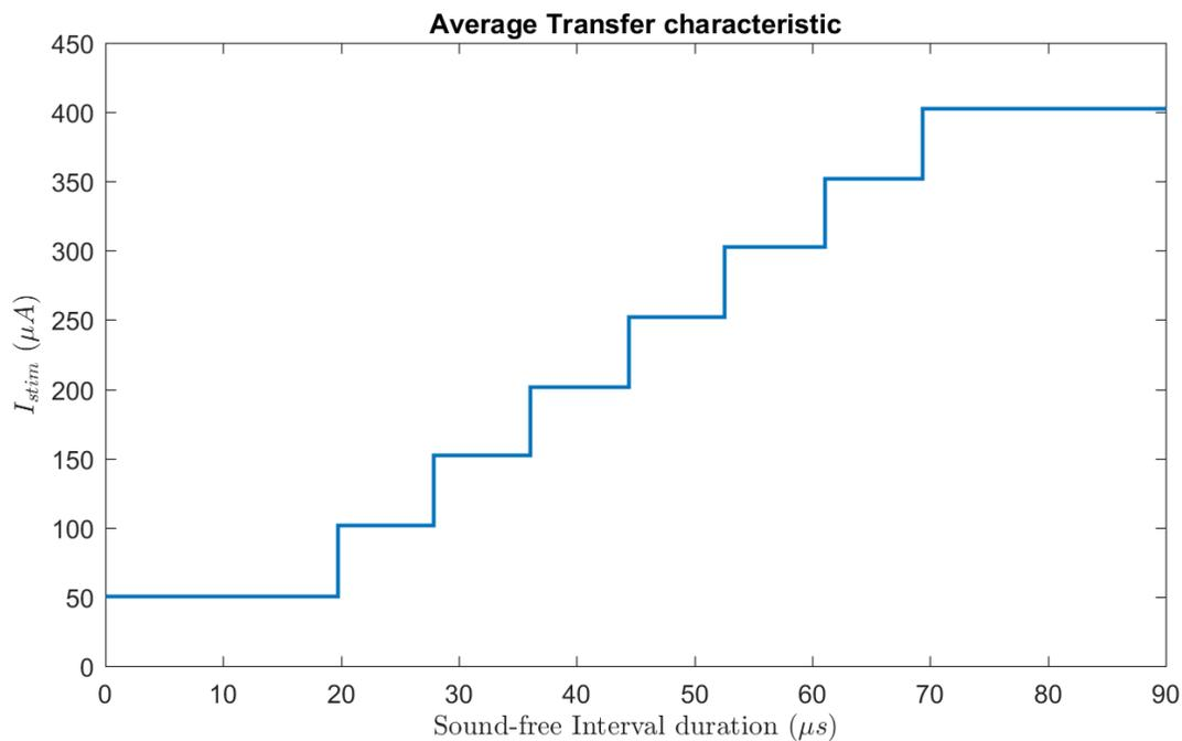
Figure 5.5: The average transfer characteristics of five chips.
