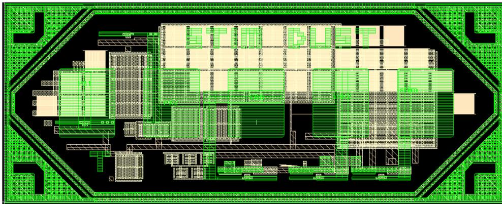
Figure 4.2: The layout showing that the chip is heavily decoupled using MIM and MOM capacitors to consolidate the structure. Green: top metal; Beige: MIM and MOM capacitors.
