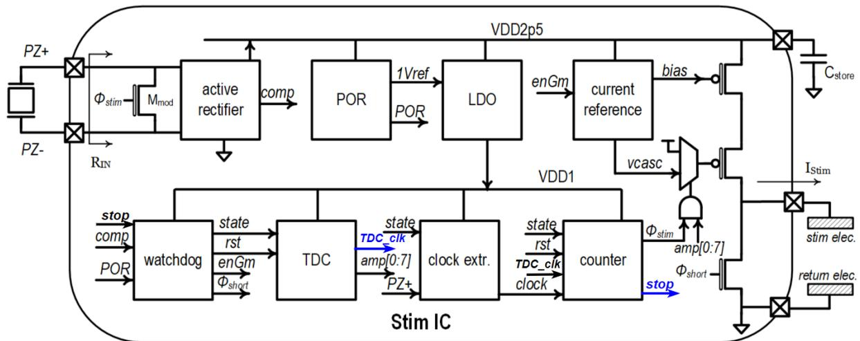
Figure 3.1: Circuit block diagram of the chip. The signals in blue are new for this chip to support the safety timer.
