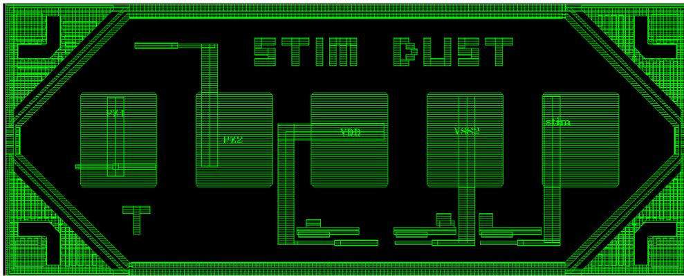
Figure 4.1: The top metal layer of the layout. The pads are evenly distributed along the center line of the layout. The structure around the pads is the sealing.
