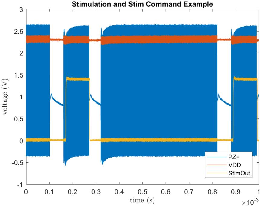
Figure 5.3: The waveform of the PZ+, VDD, and StimOut during stimulation.
