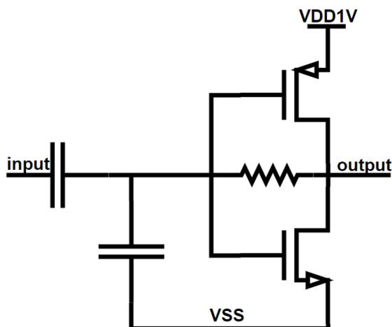
Figure 3.13: CMOS inverter in resistive feedback used to extract AC signal as clock.
