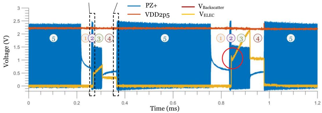
Figure 1.4: The output waveform of the previous generation StimDust [11]. The current peaking is circled in red. The amount of peaking is worst when the output current is at the maximum level.
