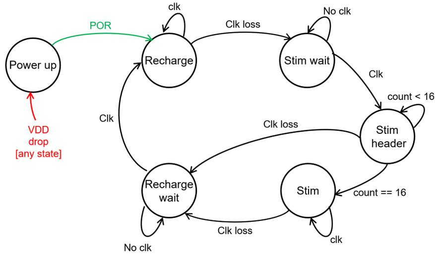
Figure 2.4: Finite state machine of the previous chip.
