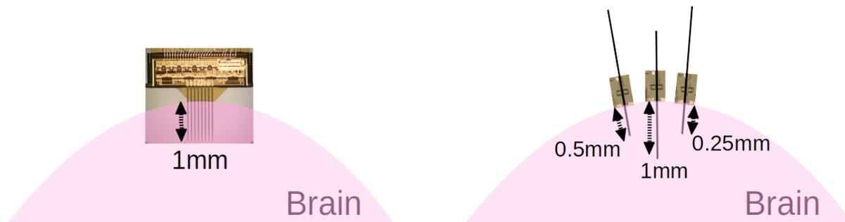
Figure 3.2: Left: Insertion of a microwire array with recording sites at a fixed relative position within the array. Right: Insertion of individual electrodes to independent depths.
