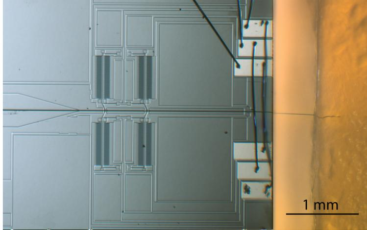
Figure 3.24: The MEMS actuator and a  $7.2\ \mu\text{m}$  diameter carbon fiber inserted approximately  $400\ \mu\text{m}$  into the agar brain phantom.
