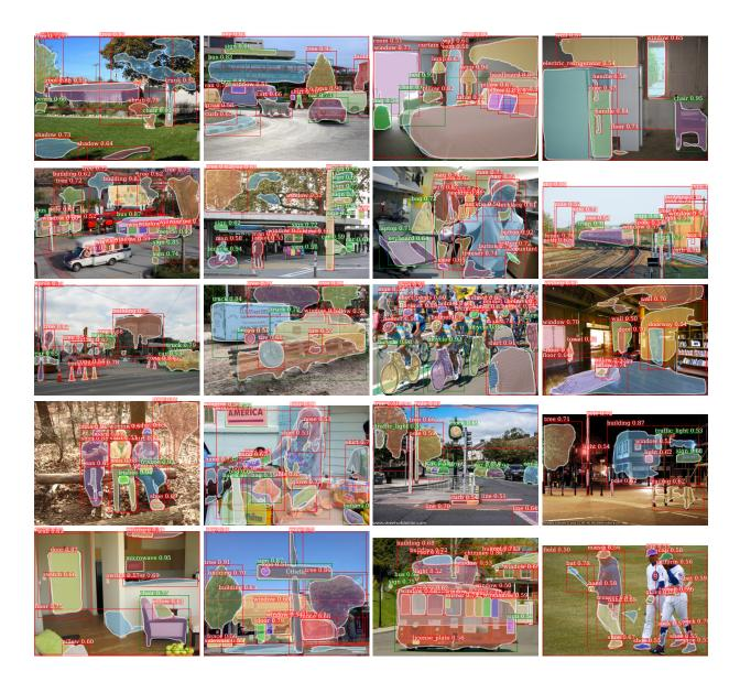
Figure 4.1: Example mask predictions from our Mask<sup>X</sup> R-CNN on 3000 classes in Visual Genome. The green boxes are the 80 classes that overlap with COCO (set A with mask training data) while the red boxes are the remaining 2920 classes not in COCO (set B without mask training data). It can be seen that our model generates reasonable mask predictions on many classes in set B. See §4 for details.
