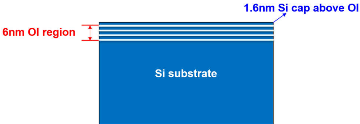
Fig. 5.2. Schematic cross-sectional view of the 6nm-thick OI region in the OI silicon wafer samples used in this work.
