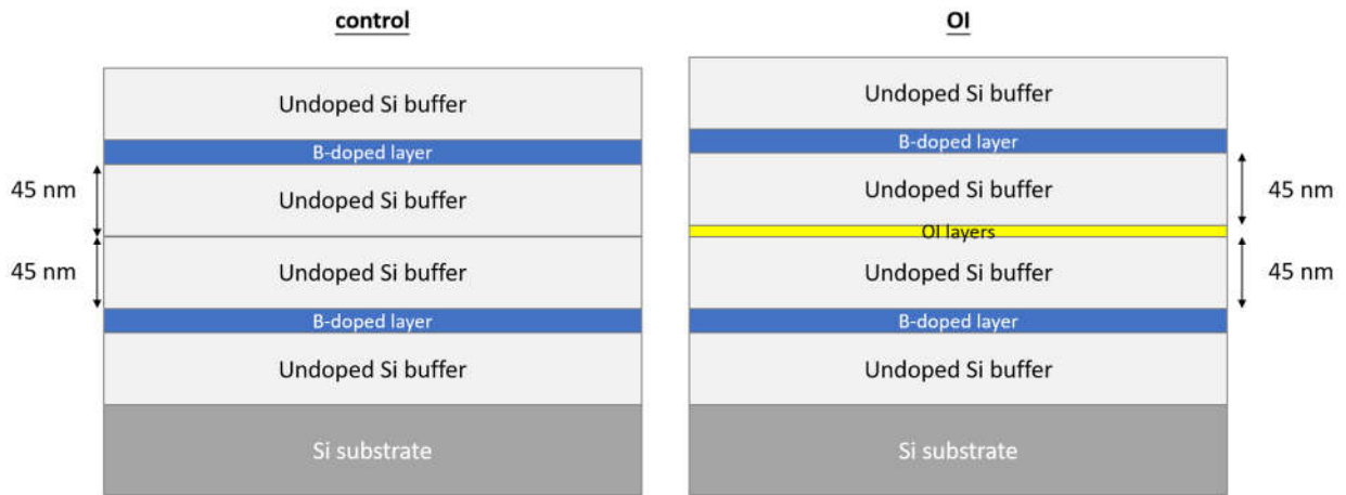
Fig. 2.13. Cross-section schematics of boron marker layers in epitaxially grown silicon samples. 6 nm thick OI layers protect the lower boron marker layer from OED.
