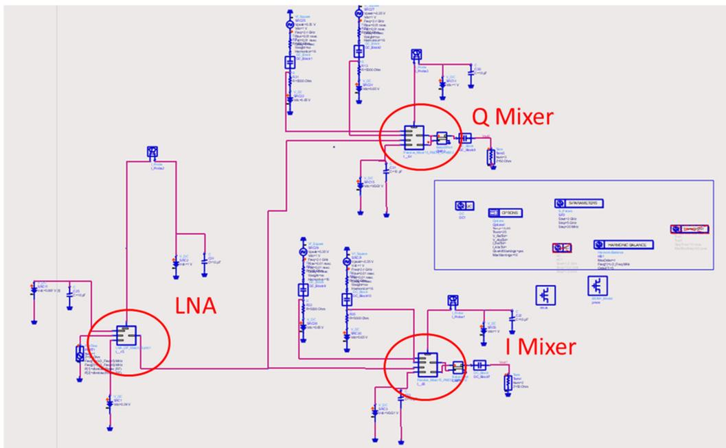
Figure 42: Receiver front end test bench
