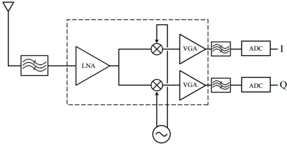
Figure 1: Block diagram of the receiver
