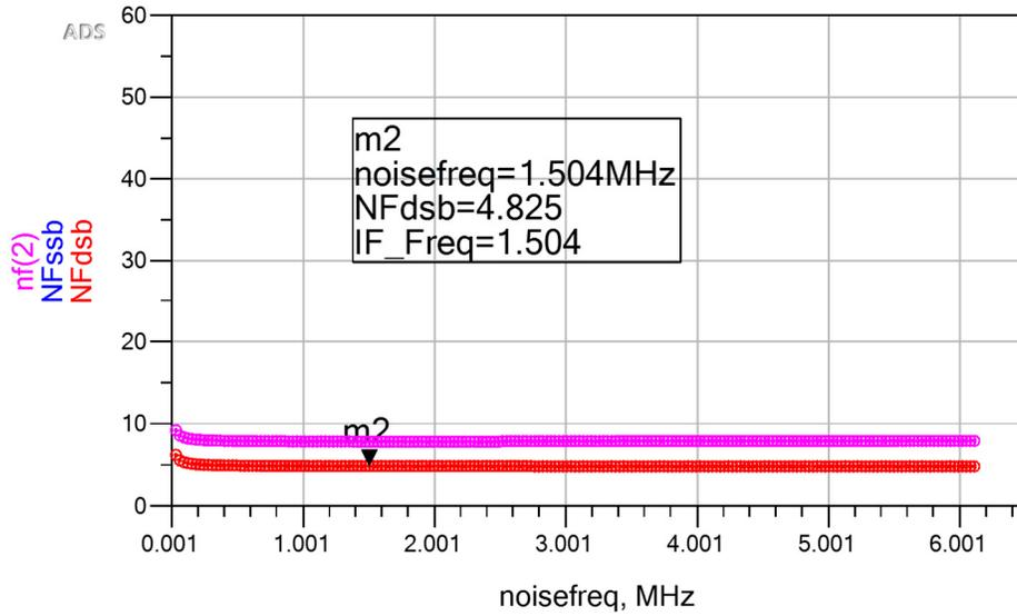
Figure 25: Noise figure of the receiver front end
