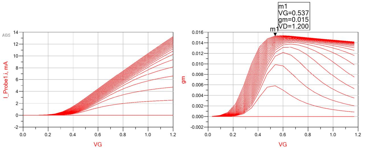
Figure 3: (left)DC IV simulations on a 1µm/65nm NMOS and (right) transconductance vs  $V_{GS}$
