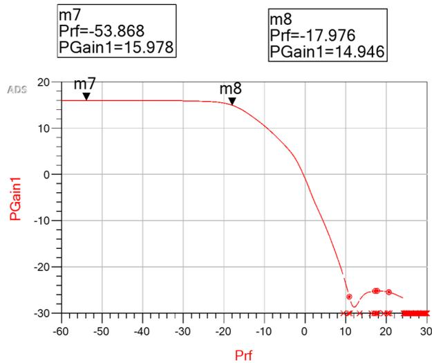
Figure 15: Gain compression of the LNA
