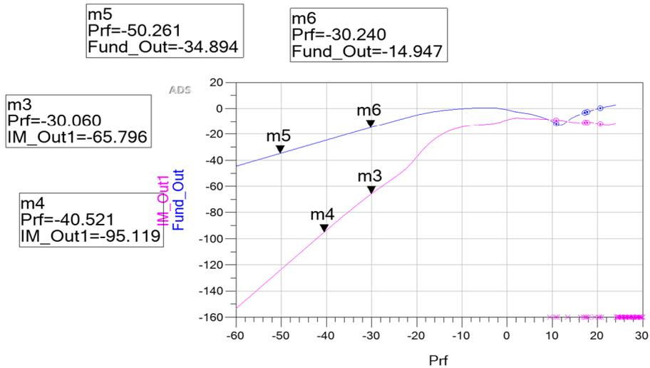
Figure 16: Third order intermodulation and fundamental v/s input power
