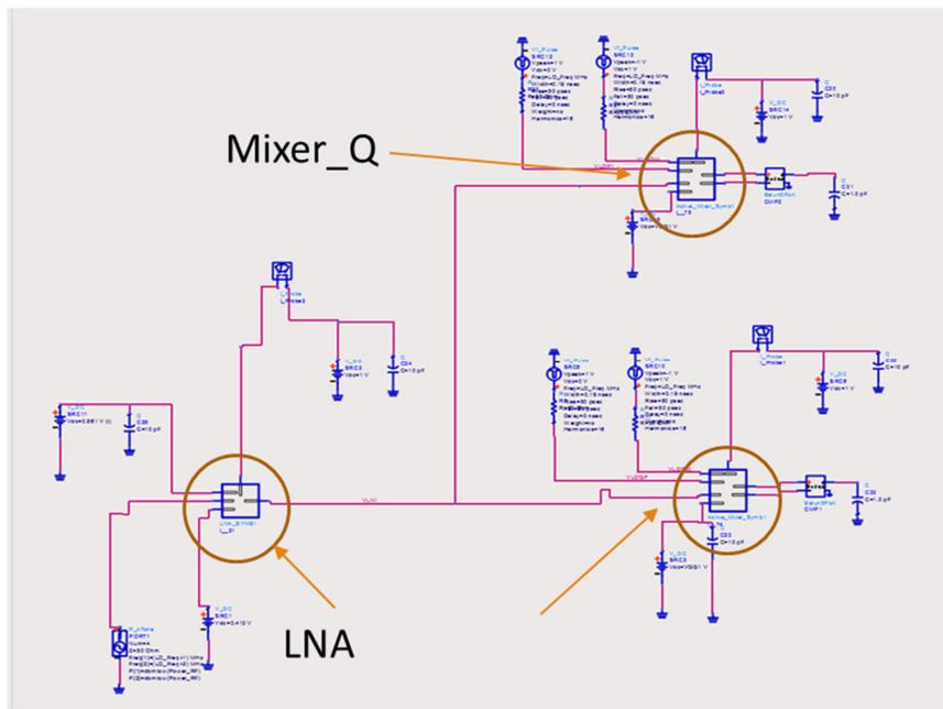
Figure 24: Receiver front end test bench
