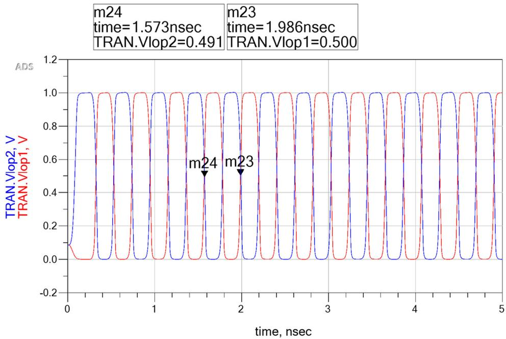
Figure 48: Transient signal at the input of the LO gate
