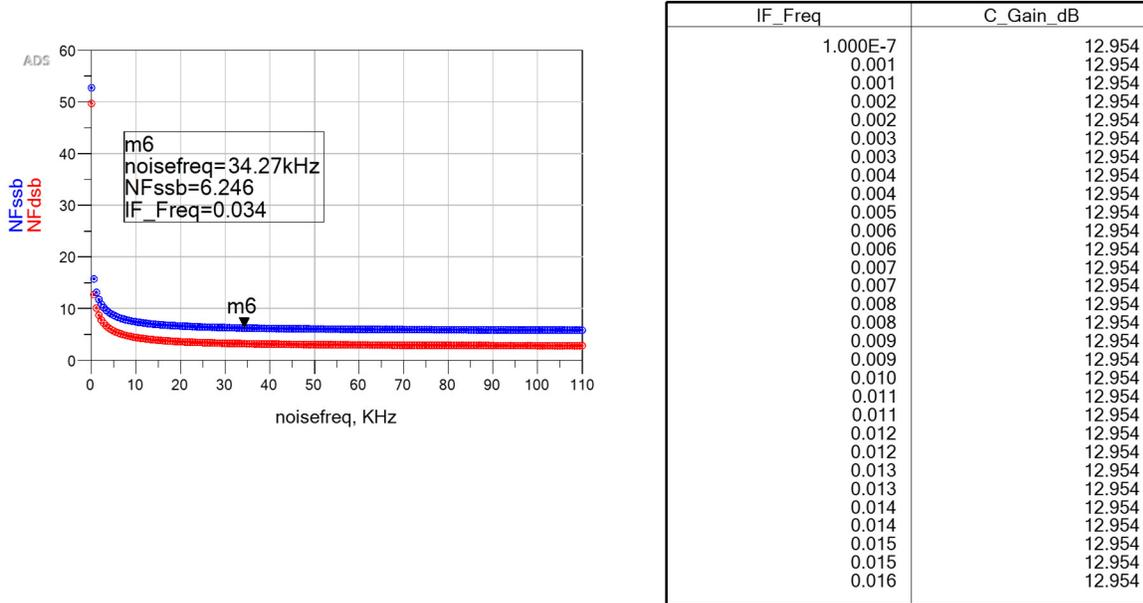
Figure 21: Active Mixer Noise Figure and Conversion Gain
