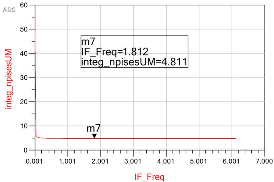
Figure 26: Integrated noise figure of the receiver
