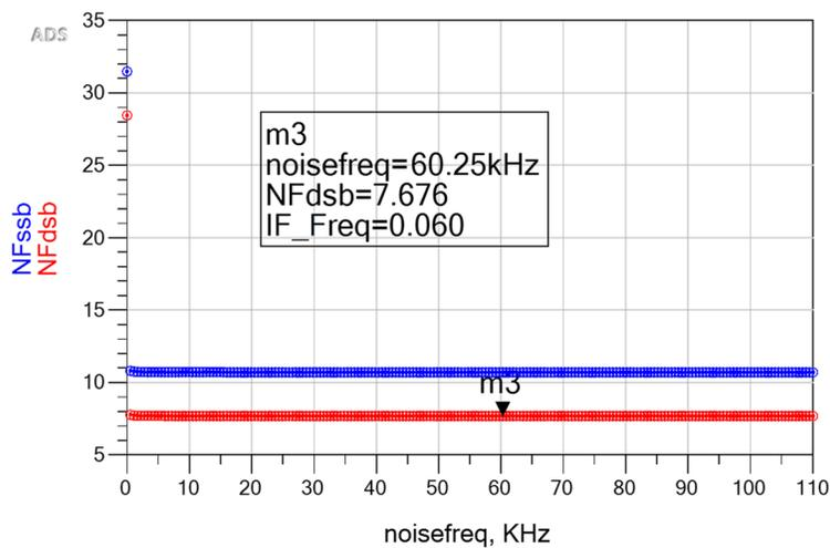
Figure 40:Passive Mixer Noise Figure
