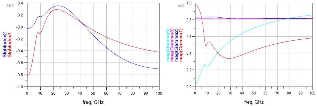
Figure 10: Stability indices for the LNA (left) and the reflection coefficients at each node(right)
