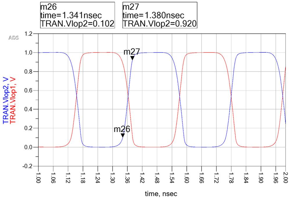
Figure 49: Square wave at the LO input showing finite rise time of 40ps
