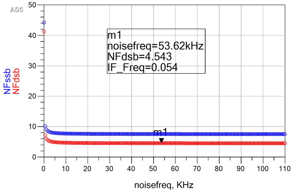
Figure 43:Noise figure of the receiver front end
