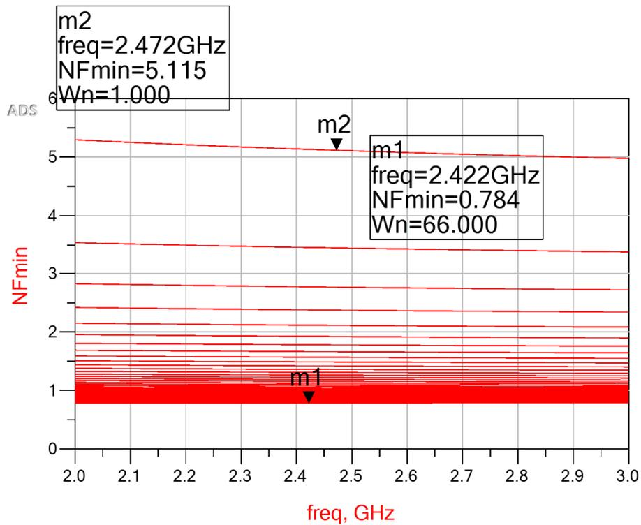
Figure 4:  $NF_{min}$  Vs Device width for dc current of 1mA and  $V_{DS} \sim 0.4V$
