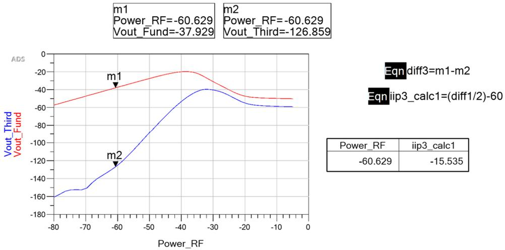
Figure 51: Third order intermodulation and fundamental output of the receiver with passive mixer and LO driver
