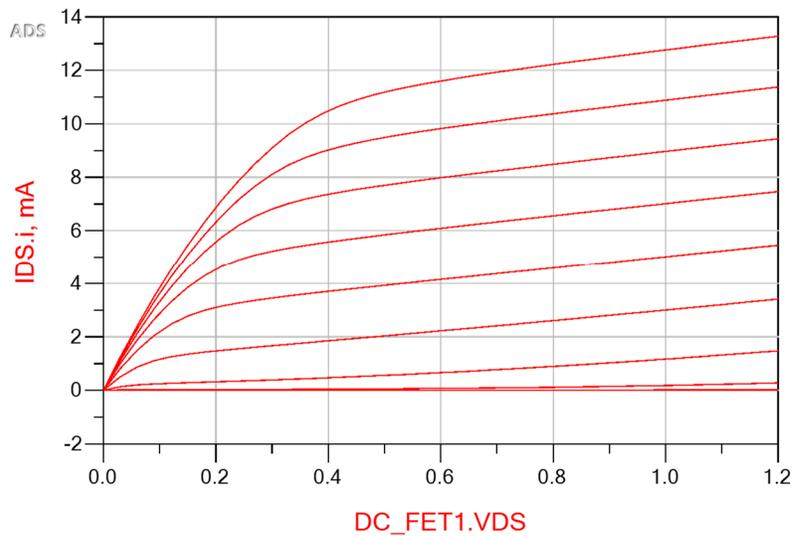
Figure 2: I-V simulations on a  $1\mu\text{m}/65\text{nm}$  NMOS
