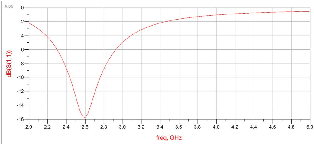
Figure 18: Input return loss( $S_{11}$ ) of the active mixer
