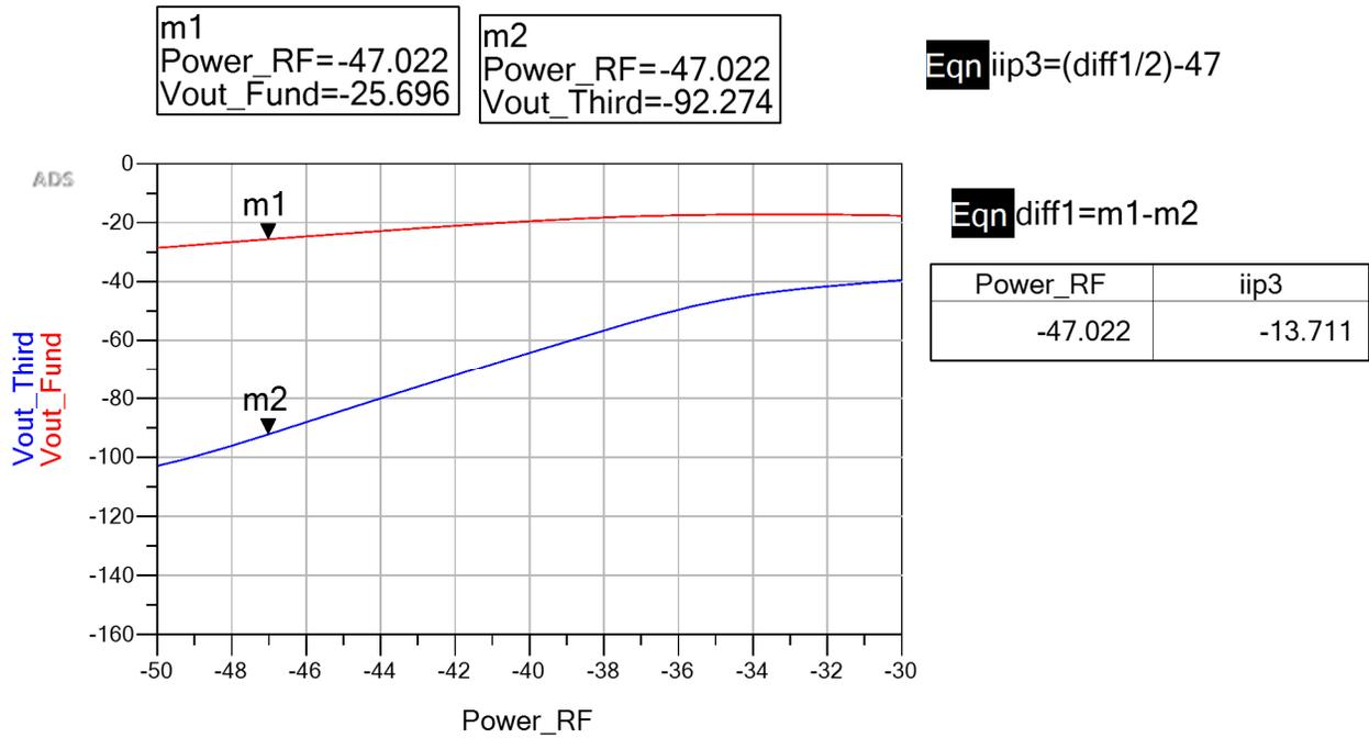
Figure 44: Receiver with passive mixer IIP3
