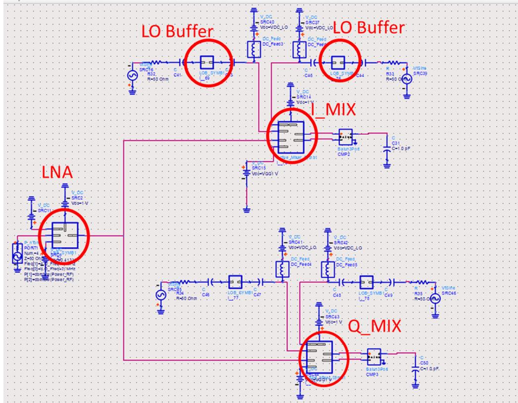
Figure 46: Receiver with LO buffer-driver integrated
