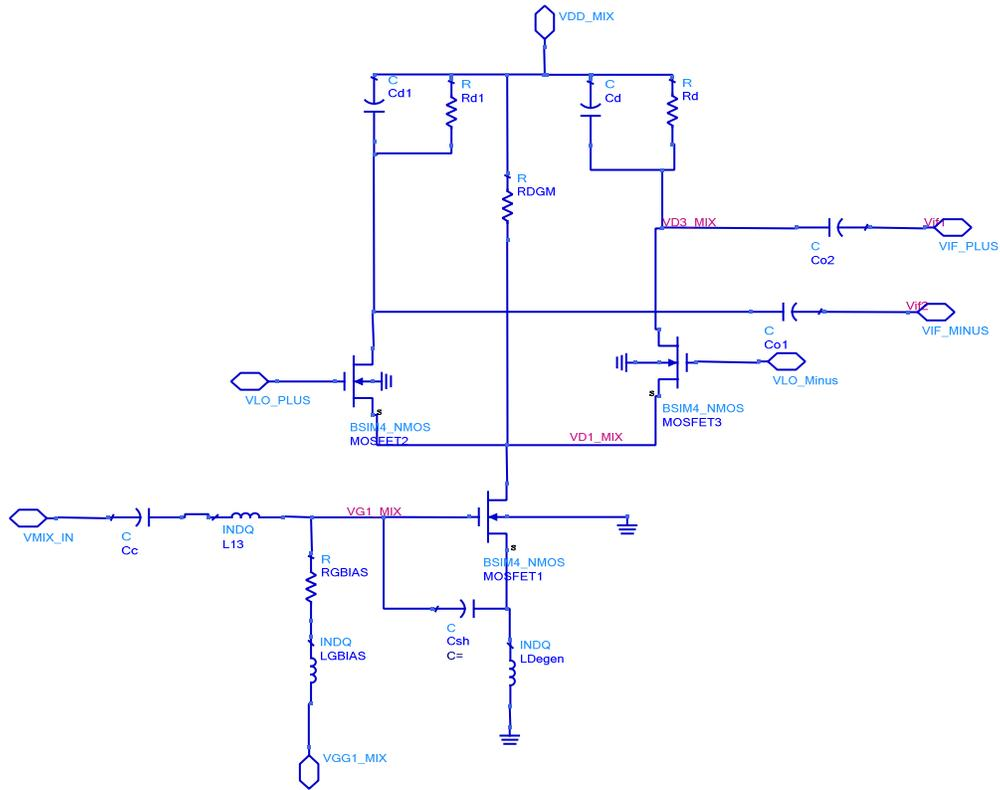
Figure 19: Active mixer schematic
