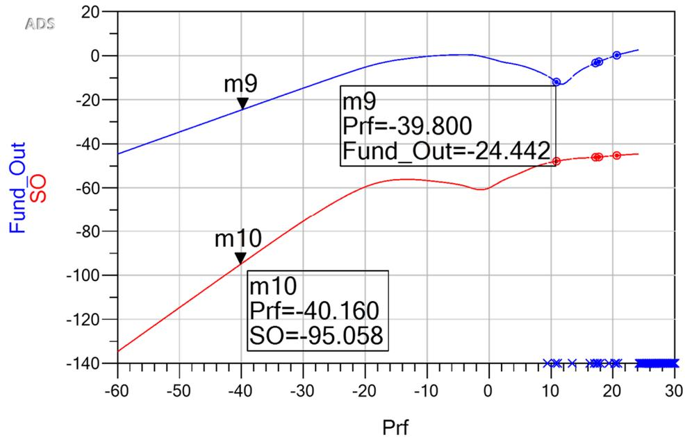
Figure 17: Second order intermodulation and fundamental v/s input power
