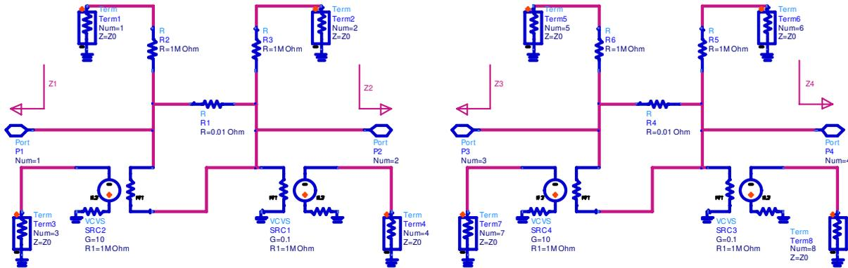
Figure 9: Schematic of the S-probe pair
