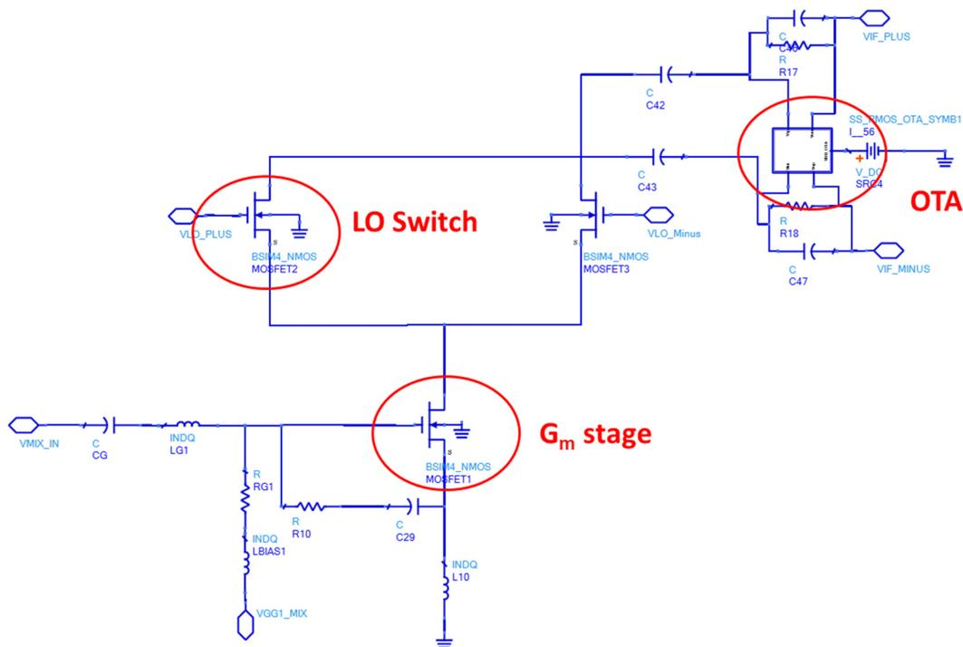
Figure 32: Passive mixer schematic
