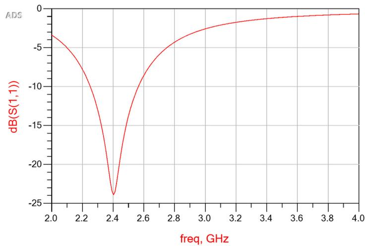
Figure 8: Input return loss of the LNA
