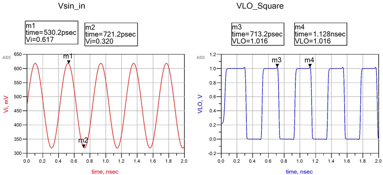
Figure 30: 300mV sinusoidal input(left) and 1V square wave output(right) from the LO buffer-driver circuit
