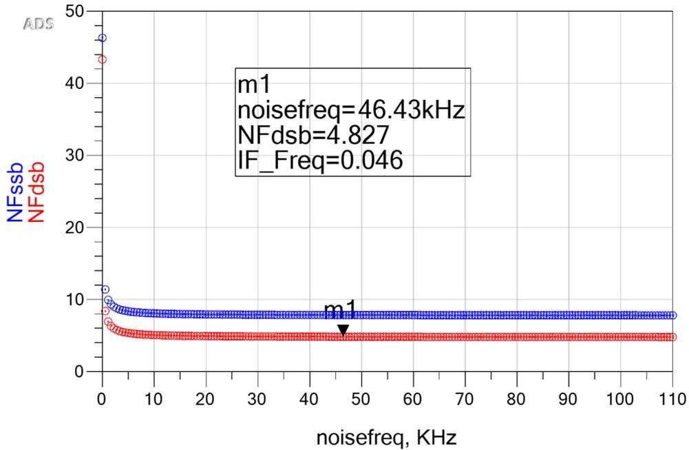
Figure 50: Noise figure of receiver with passive mixer (with LO buffer integrated)
