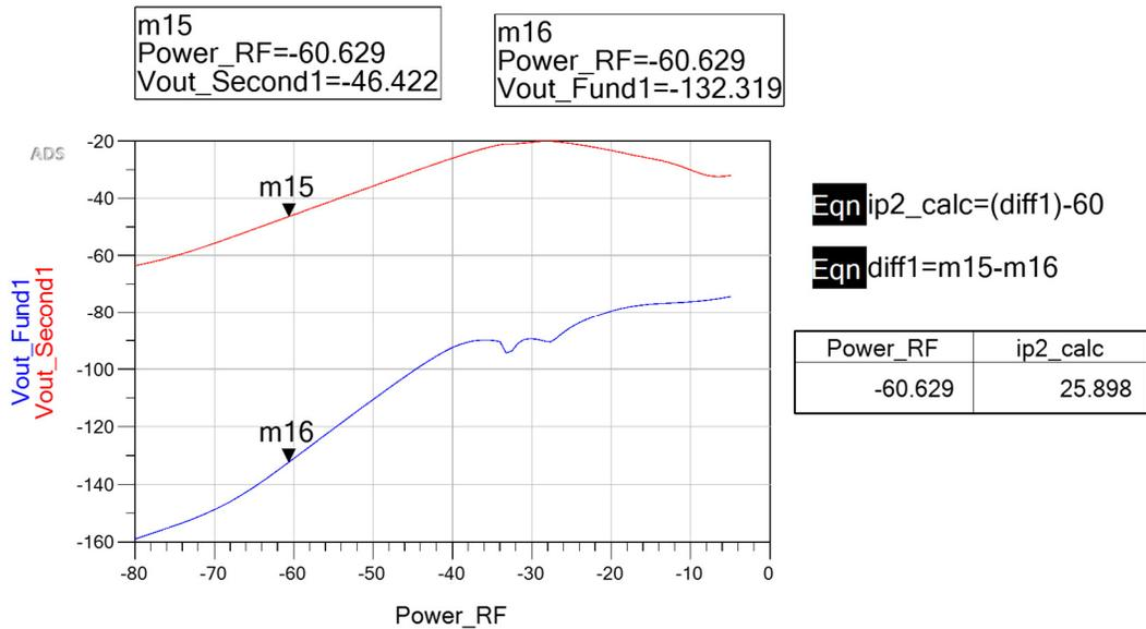
Figure 45: Simulated IIP2 of the receiver with passive mixer
