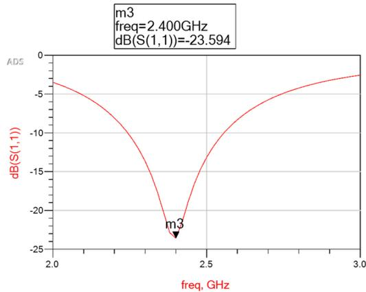
Figure 23: optimized input match for the active mixer
