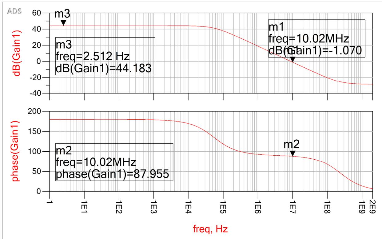
Figure 37: Gain and Phase Margin of the OTA used in the TIA
