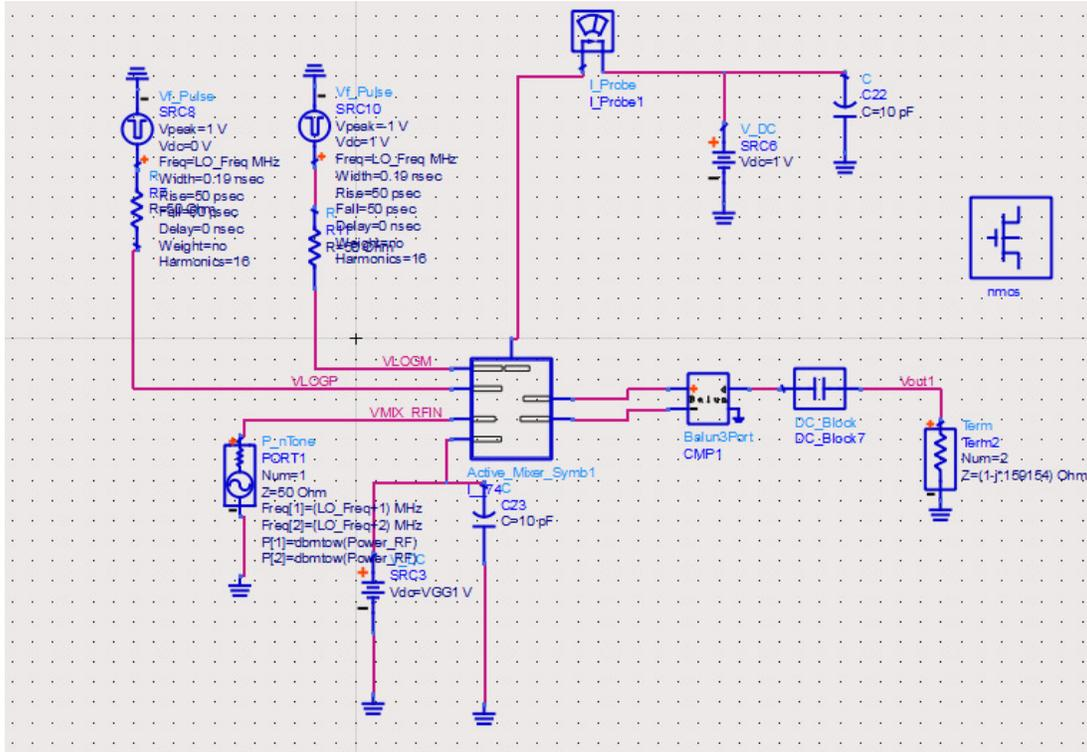
Figure 20: Active mixer test bench
