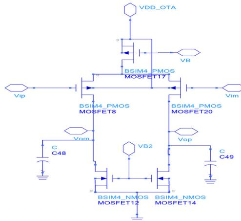
Figure 33: Fully differential OTA topology
