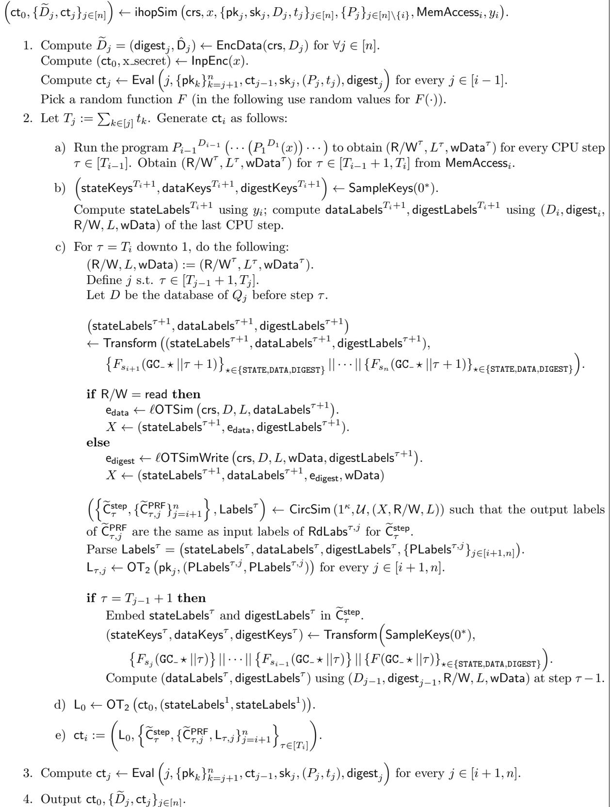
Figure 4.10: Simulator for multi-hop RAM.
