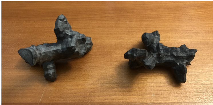
Figure 3.9: Adversarial Intersected Cylinder Objects for Physical Experiments. These objects were generated by the CEM + GAN method.
