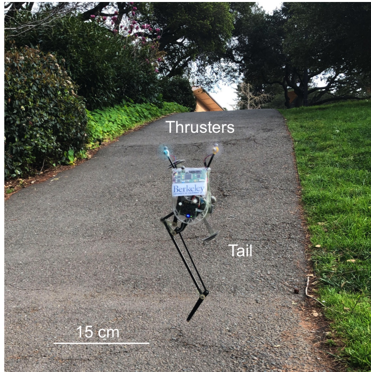
Figure 3.1: Salto-1P jumps outdoors without external sensing.
