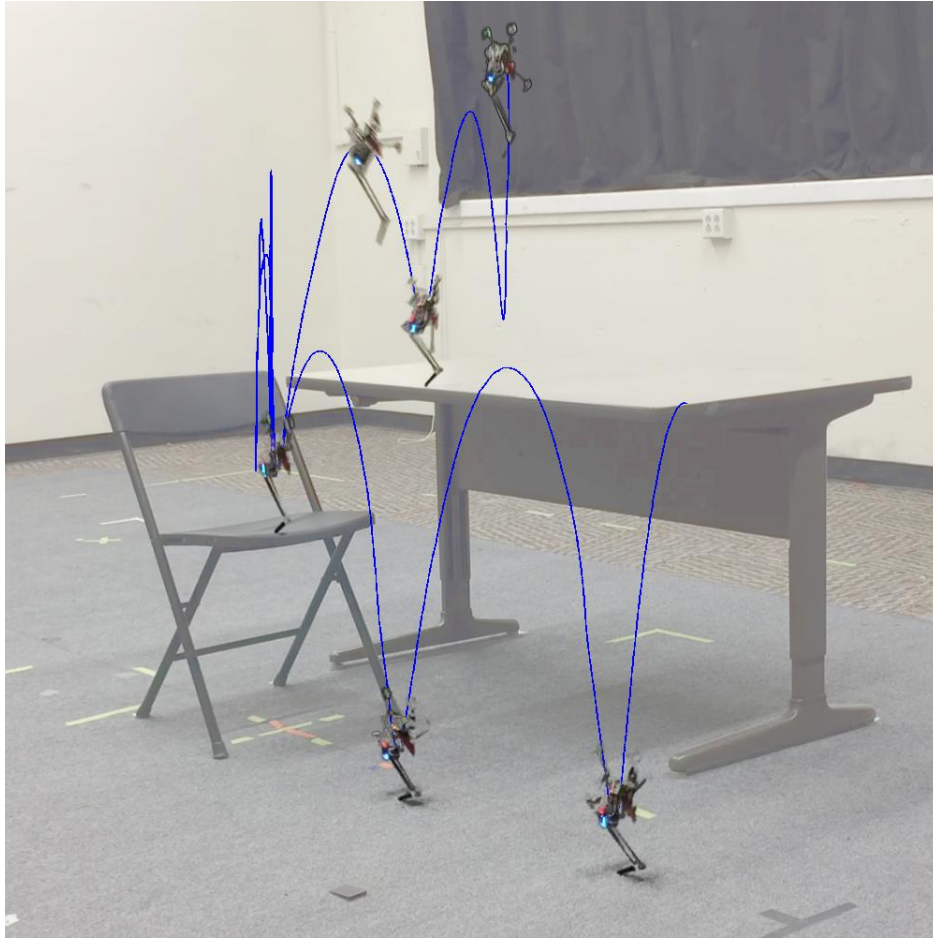
Figure 2.8: The robot jumps up onto a chair and desk (trajectory in blue), then back down (not shown here, but shown in Fig. 2.9).
