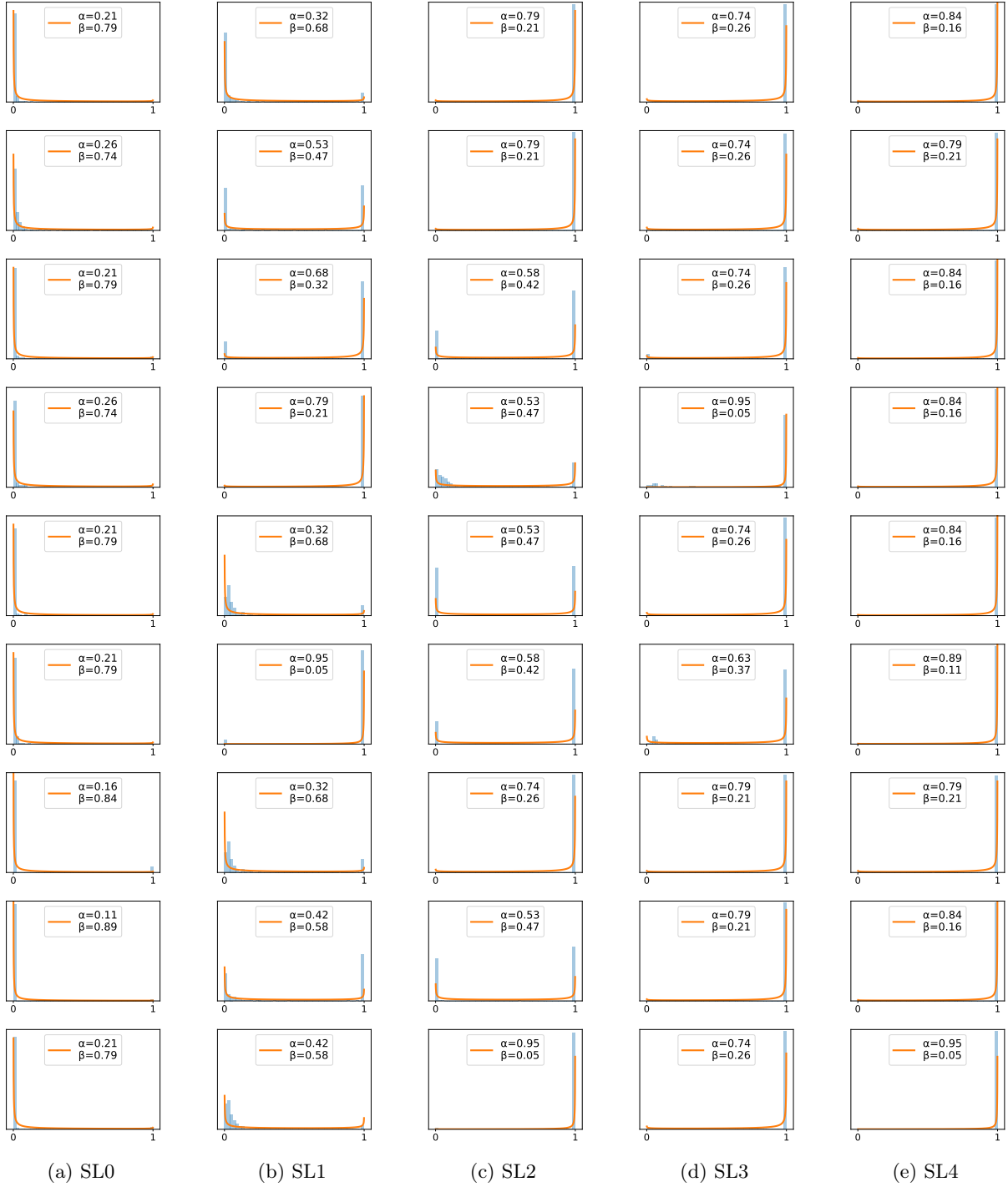
Figure B.1: Histograms showing the spread of trained (with \rho = 0.2 ) DT models' predictions on a selected numbers of data examples from the chiller dataset, and a fitted beta distribution \mathcal{B}(\alpha, \beta) for each example.
