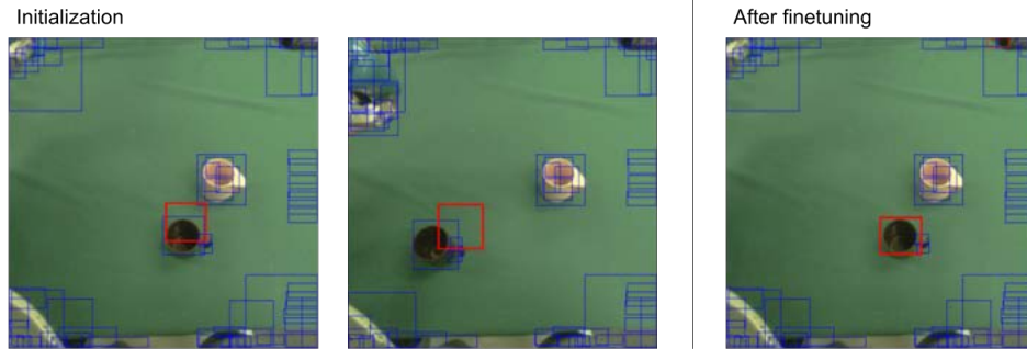
(a) Left: The soft attention from just training on the brown mug is shown in red. Right: The soft attention after finetuning on demonstrations where the pink mug is present. When initialized on only the brown mug, the attention is sensitive to "mug" features, and therefore can be distracted by the pink mug. After adding demonstrations of pouring into the brown mug with the pink mug in the background and finetuning, the attention has locked on to just the brown mug. The blue squares show the task-independent attention.
