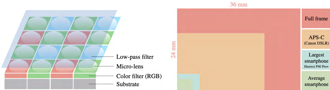
Figure 1.3: Left: A simple diagram of Bayer sensor used in most CMOS sensors. Incident light is focused by the micro-lenses and filtered by the green, red and blue color filters. Low-pass filter, or Anti-aliasing filter (AA filter) alleviates moiré or other high-frequency artifacts, but undesirably blurred out details. Many modern cameras have thus left the AA filter out. Right: Image sensor size comparison. Even the largest smartphone sensor is small in size, compared to conventional large cameras ( e.g. DSLR). This causes great challenges to produce good quality imagery on small cameras ( e.g. smartphones).
