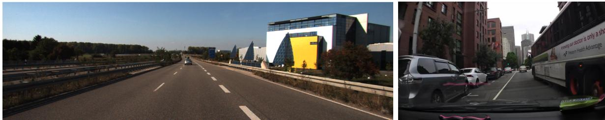
Figure 3.1: Comparison of a KITTI image (left) and a BDD dashcam image (right). The BDD image features a narrower field of view and more surrounding moving objects, which makes the monocular visual odometry problem much more challenging than that in the KITTI dataset.
