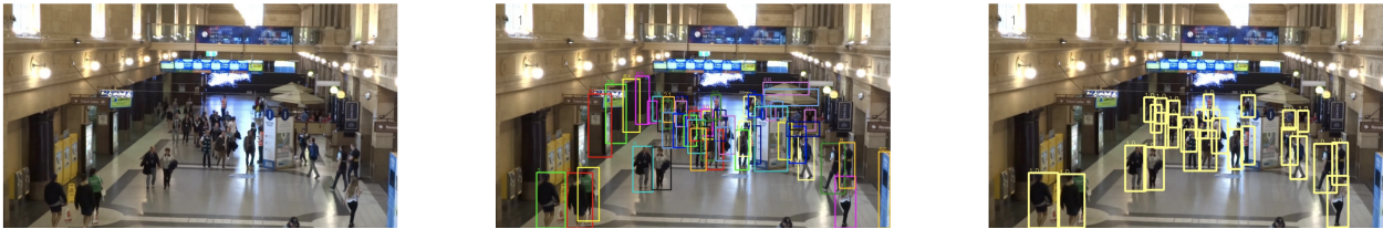
Figure 3.1: A sample sequence from the MOT20 dataset. Left: original video frame; middle: frame with labeled ground truth bounding boxes, right: Faster R-CNN detections. Image adapted from MOT20 paper [10].
