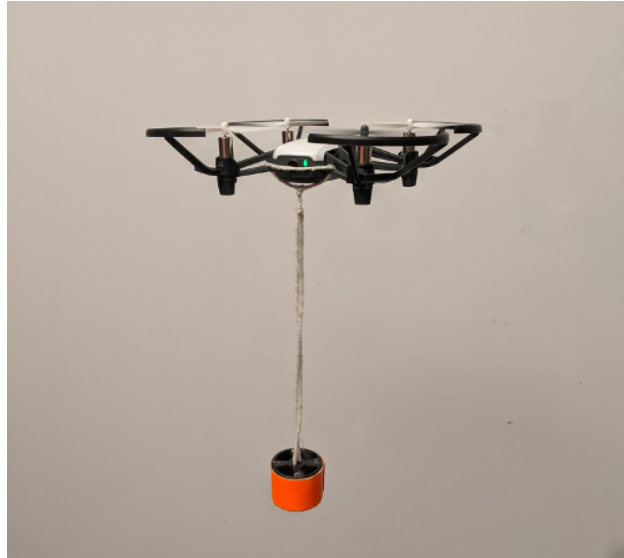
Figure 4.1: DJI Tello with suspended payload.
