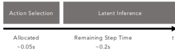
Figure 4.4: Visual diagram for the time split of one control loop. We minimize action selection time (reactivity) and thereby maximize latent inference time (adaptability)
