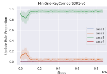
Figure 5.6: Our learned algorithm, DQNClipped, can be broken down into four update rules where each rule is active under certain conditions. Case 3 corresponds to normal TD learning while case 2 corresponds to minimizing the Q-values. Case 2 is more active in the beginning when value overestimation is a problem and then becomes less active as it is no longer needed.
