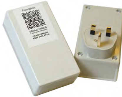
(b) PowerWatch sensors.
