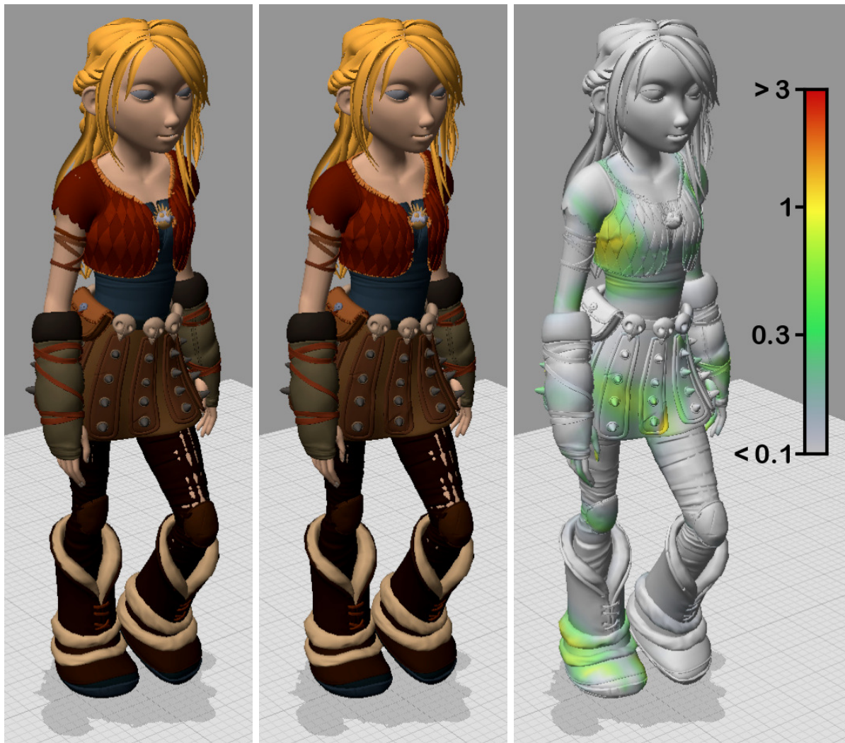
Figure 2.4: Side-by-side comparison of the ground truth mesh (left) and the approximation (center). The vertices of the approximated mesh are colored to indicate the per-vertex distance error (right). Errors above and below the range of the scale are clamped to the ends of the color range. All distances are measured in centimeters. 1
