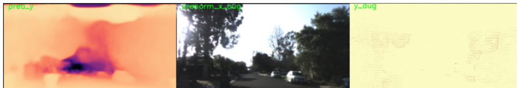
Figure 4: Qualitative Performance of PixelBins; please see Supplementary Materials for more qualitative visualizations on test set. Left: PixelBins depth map prediction. Middle: Ground truth input image. Right: Ground truth point cloud. Note that the ground truth point cloud is sparse; the fine-detail is best viewed by zooming in on an electronic copy.
