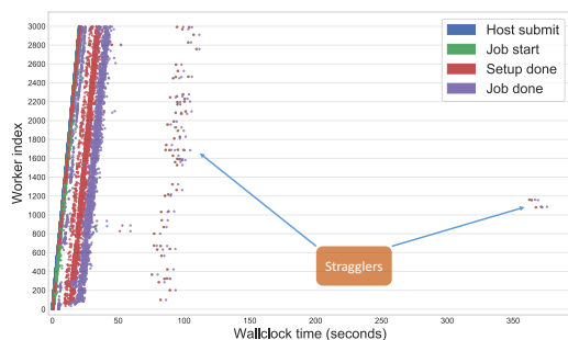
(a) Job times for 3000 AWS Lambda nodes in one trial. The median job time is 40 seconds, and \sim 5\% of the nodes take 100 seconds, and two nodes take as much as 375 seconds for the same job.
