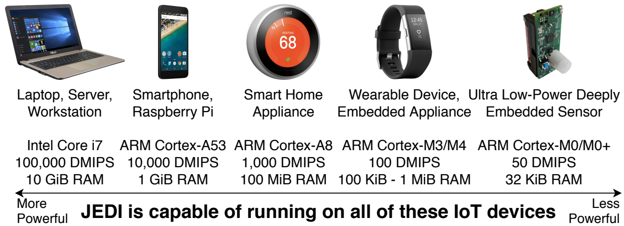
Figure 6.1: IoT comprises a diverse set of devices, which span more than four orders of magnitude of computing power (estimated in Dhrystone MIPS). 1
