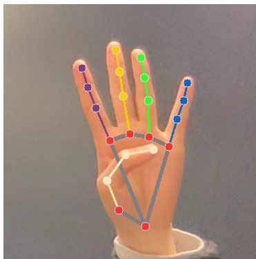
Figure 2.4: The thumb state is 'CLOSE' and all other finger states are 'OPEN' for the 'four' gesture shown when using relative position gesture recognition.
