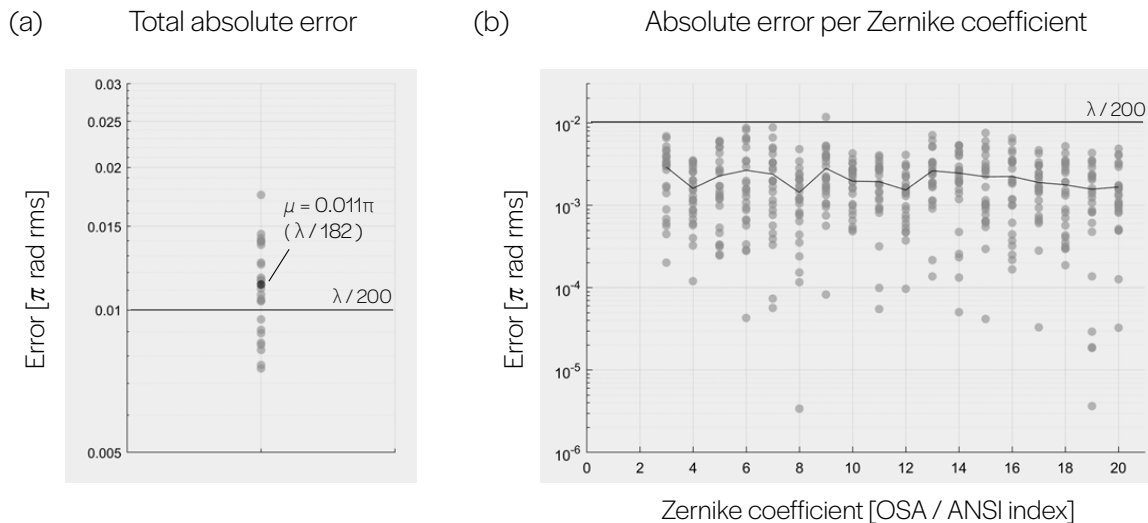
Figure 3.15: Total reconstruction error and error per coefficient. (a) Total reconstruction error for 25 datasets of simulated speckle images for imaging systems with aberrations of magnitude 0.2\pi rad rms (from 100 initializations). (b) Reconstruction error per coefficient for the same set of simulated reconstructions.
