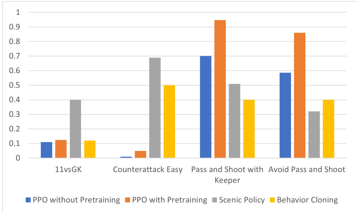
Figure 3.2: Bar chart comparing the performance of agents trained with and without demonstration data. The first two columns represent the average goal difference of RL agents without pretraining and with pretraining. The third and fourth columns show the performance of the semi-expert Scenic policy and the behavior-cloned agents. The first two scenarios, 11vsGK and Counterattack Easy, had environment-controlled teammates, while the last two scenarios, Pass and Shoot with Keeper and Avoid Pass and Shoot, had all relevant players controlled by RL agents.
