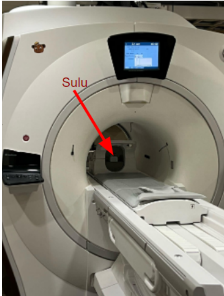
Figure 3.7: Image of SC \mu M Sulu development board in the bore of a 3T MRI machine immediately prior to testing performance during a performance test.
