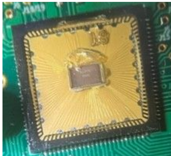
Figure 2.5: Damaged packaged SCμM chip on Sulu due to adding through-hole components with a soldering iron. Connections to this SCμM chip have been irreparably damaged and Sulu is unable to get SCμM to boot.
