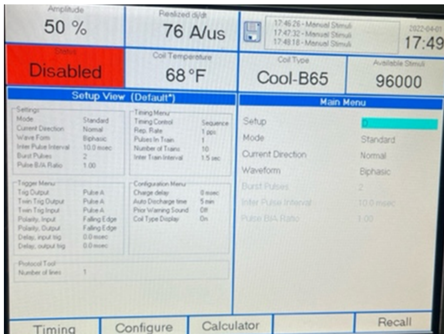
Figure 3.10: MagPro X100 TMS machine and Cool-B65 coil used for TMS tests (top). Example of settings of TMS MagPro X100 machine during the TMS test (bottom). Single biphasic pulses initiated manually on the coil made up the recent tests were administered before this photo was taken, as demonstrated by the upper right of the display.
