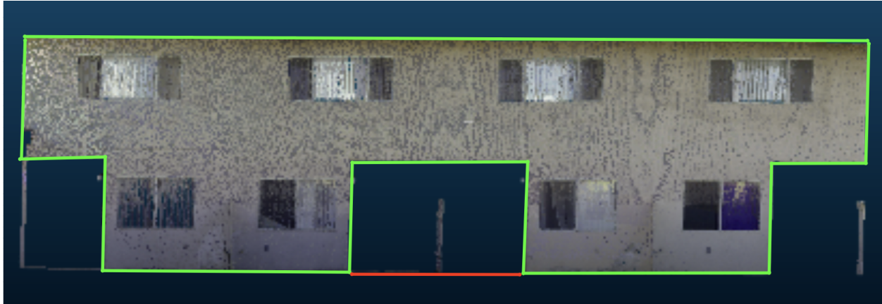
Figure 3.6.: Example of edge validation: red edges are removed and green ones are kept.
