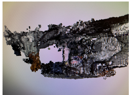
Figure 4.5: Point cloud generated by the ZED2 for Scene 2
