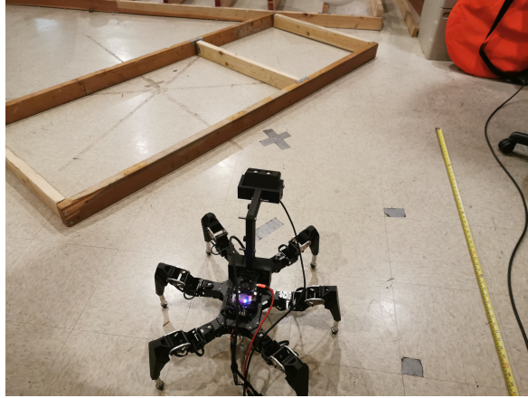
Figure 2.22: Test 5: hexapod starts at 1m from 60^\circ oriented joist. The resulting grid map images and line detections for this experiment are shown in Appendix E. Demo video .
