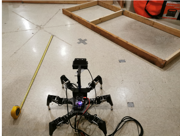
Figure 2.21: Test 4: hexapod starts at 1m from 45^\circ oriented joist. The resulting grid map images and line detections for this experiment are shown in Appendix D. Demo video .
