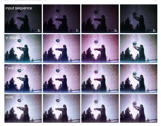
Figure 7.7: **Video Results**. Results on noisy video clip, showing performance over time for a video taken at 10fps in 0.6 mlx. Our method achieves better temporal consistency than V-BM4D or the pretrained FastDVDnet, and also has fewer artifacts within each frame. See Appendix A.3 for full video clips. (Digital zoom recommended.)
