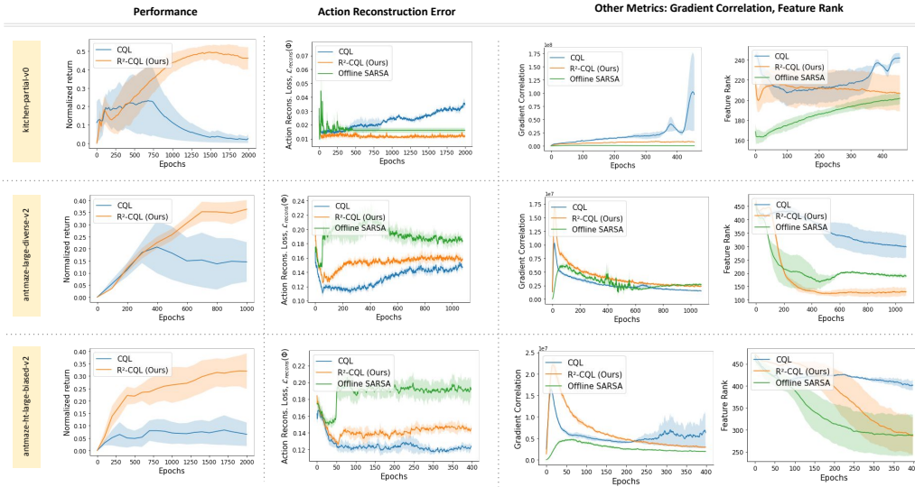
Figure 5: Performance and metrics of R^2 -CQL vs regular CQL, in comparison with SARSA. Observe that measuring of closeness of the reconstruction error on the dataset actions (Metric A.1) to the corresponding value for SARSA is able to accurately predict the performance trends, while other prior metrics may not.
