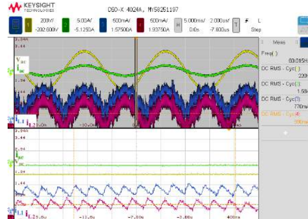
Figure 6.27: Typical current waveforms of the interleaved FCML, PFC mode from 240 V ac to 400 V dc , 375 W.
