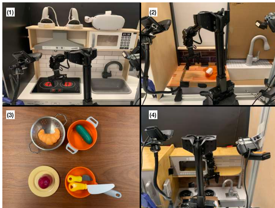
Figure D.1: Setup Overview: Following [45], we use a toykitchen setup described in that prior work for our experiments. This utilizes a 6-DoF WidowX 250 robot. (1): Held-out toykitchen used for experiments in Scenario 3 (denoted “toykitchen 6”), (2): Re-targeting toykitchen used for experiments in Scenario 2 (denoted “toykitchen 2”), (3): target objects used in the experiments of scenario 3., (4): the held-out kitchen setup used for door opening (“toykitchen 1”).
