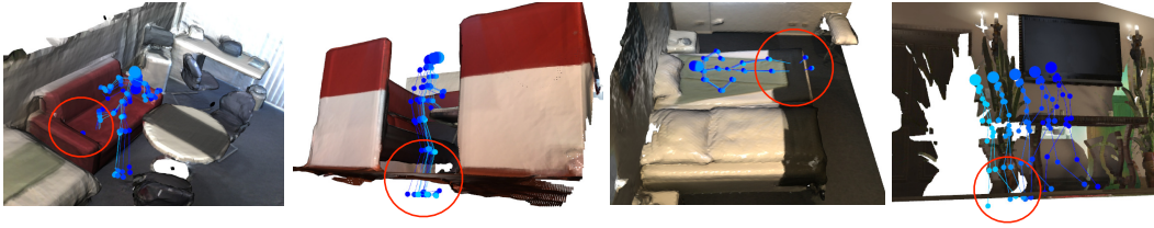
Figure 3.9: Visualization of failure cases. In each red circle area, we observe the intersection between the human feet and the 3D mesh, e.g., the bed.
