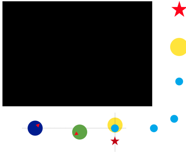
Figure 3.9: The dark blue dot represents the robot’s current position, the light blue circles represent its waypoints, the small dark red star represents its local goal, and the large bright red star represents its final goal position. The black box represents a corner, the yellow circles represent stationary objects, and the green circle represents a human. Notice that the robot’s first waypoint is in the same location as of one of the objects, so the local goal is shifted to the right side of the object with respect to the robot.
