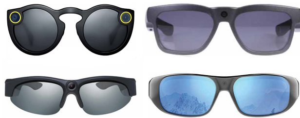
Figure 4.3: Examples of camera glasses, Friendscope’s target devices. Bipat et al. (Bipat et al., 2019) defined these as lightweight, screenless sunglasses with a very limited set of hardware, typically including a camera, microphone button, and LEDs. These devices are very different from smartglasses, which are more feature-rich and often heavier. Top left: Spectacles (Snap, Inc., 2018). Top right: Kestral Pro (Zetronix Corporation, 2019). Bottom left: zShades (Zetronix Corporation, 2017). Bottom right: OhO Waterproof Video Sunglasses (OhO sunshine, 2018).
