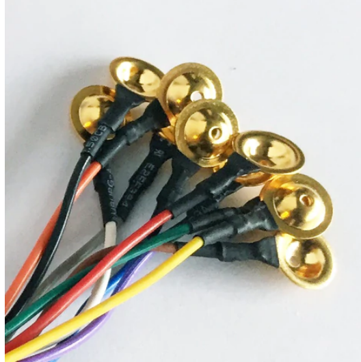
Figure 2.1: Gold-plated cup electrodes used for capturing EMG.
