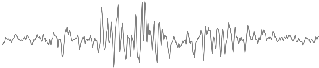
Figure 1.2: The electrical pulse from a single motor unit action potential.
