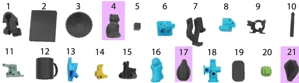
Figure 3.4: The 21 adversarial objects used in the grasp dataset collected by Danielczuk et al. [8], where analytic grasp models perform poorly. Each object is sampled with 25 test grasps, 5 trials per grasp. The training object set (cat, pear, vase) for our experiments is highlighted in purple.
