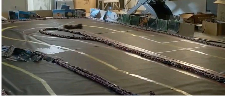
Figure 8.2: Observing human driving behavior on one-tenth scale vehicle in motion-capture track for the Robot Autonomous Racing (ROAR) project for constraint inference research as in Chapter 2
