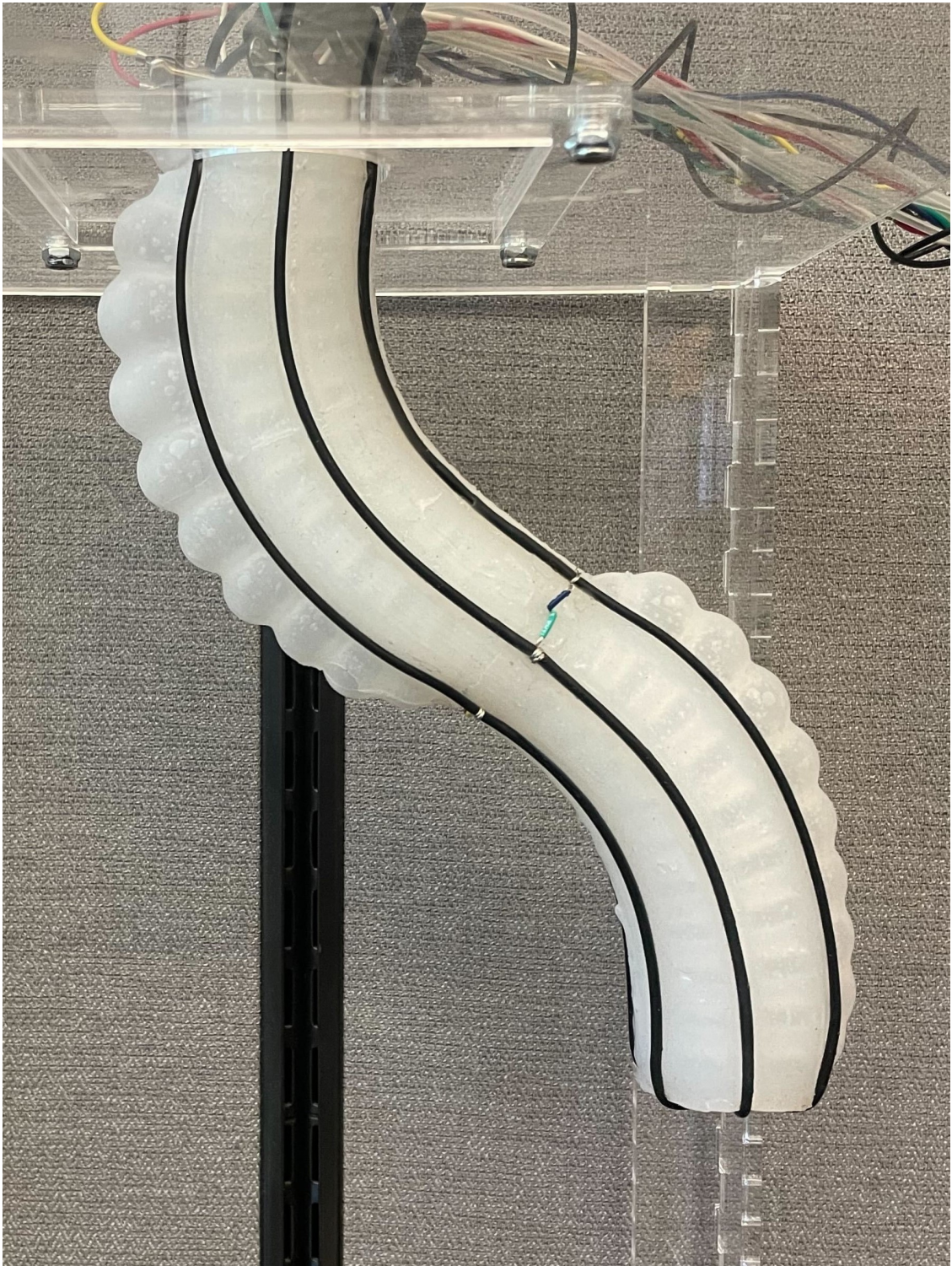
Figure 10: Complete soft robotic tentacle.
