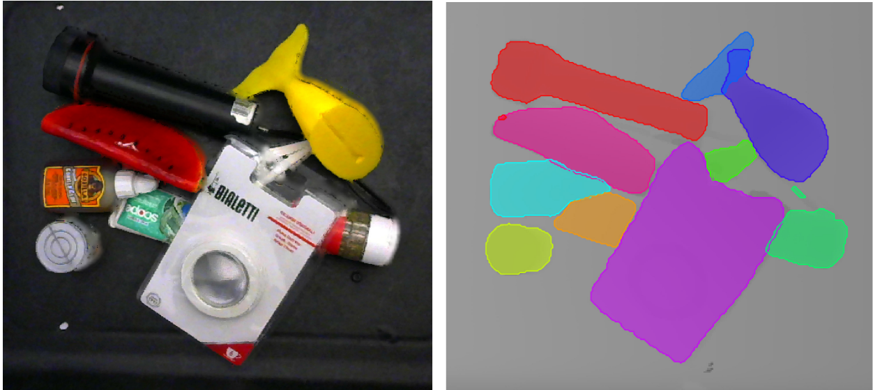
Figure 5.1: Color image (left) and depth image segmented by SD Mask R-CNN (right) for a heap of objects. Despite clutter, occlusions, and complex geometries, SD Mask R-CNN is able to correctly mask each of the objects.
