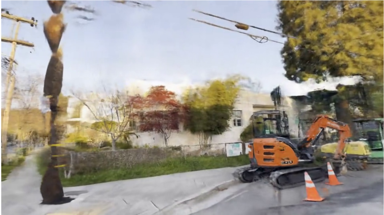
Figure 5.2: Failure Case: If the initial K -Planes has learned incorrect static geometry, it will not be corrected in the distilled LoopNeRF model, resulting in the same artifacting. See the discontinuities on the utility pole and the ghosting artifacts near the traffic cones.
