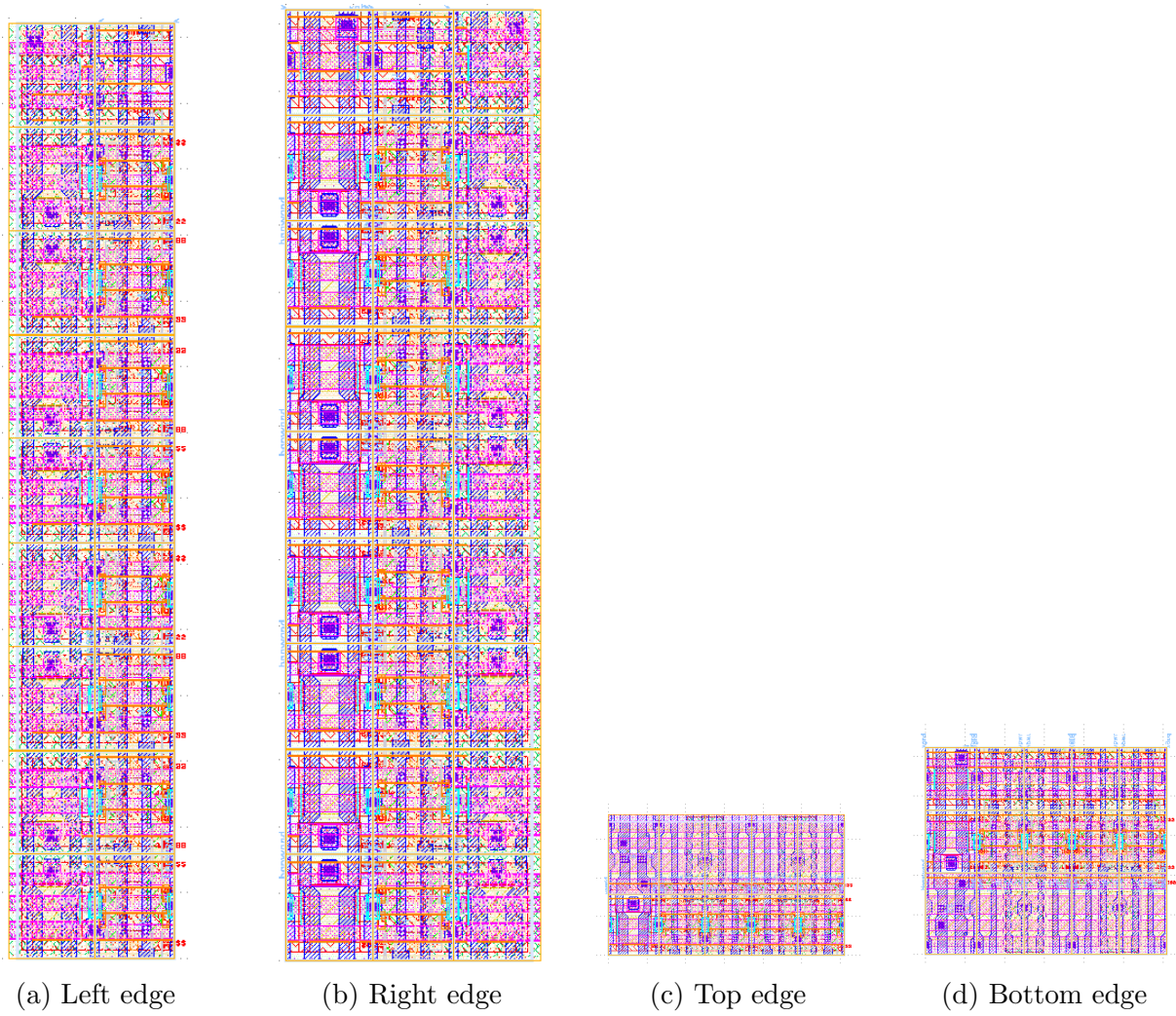
Figure 3.6: The four edge ninepatch cells for an SRAM bitcell array.
