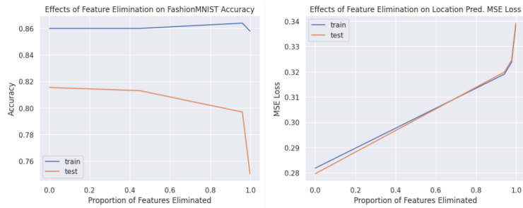
Figure 9: Model performance as a function of the proportion of features eliminated for FashionMNIST classification task and earthquake location prediction. Feature elimination is very effective for the classification task as the elimination of 90% of the model’s features leads to an accuracy drop of approx. 2%. The location prediction results are more modest as 30% feature elimination leads to a 1.5e-2 increase in MSE.
