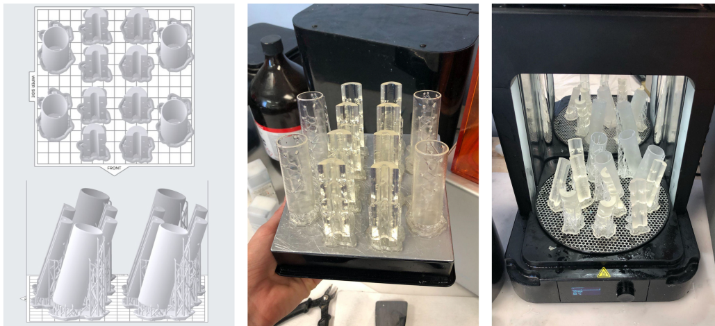
Figure 4.3: The cable traps were created by 3D printing formers on which copper tape was applied. The left image shows the modeled formers in the 3D printer software, the middle image shows them after 3D printing, and the right image shows them after UV curing [2].
